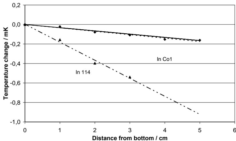
**Figure 5.** Temperature distribution along the thermometer wells during freezing (IMGC 2003). The full line represents the calculated hydrostatic effect.
