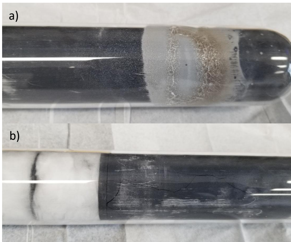
Figure 1. Picture of the NRC K9 Zn reference cell showing damage to the quartz envelope (a) and cracks in the graphite crucible (b).
