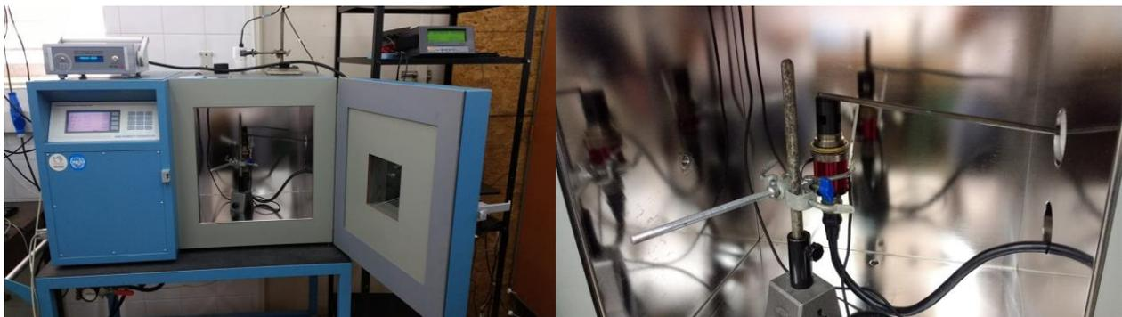
Figure 3 – Transfer Standard Sensor Inside of the Chamber of INTI Primary Generator
