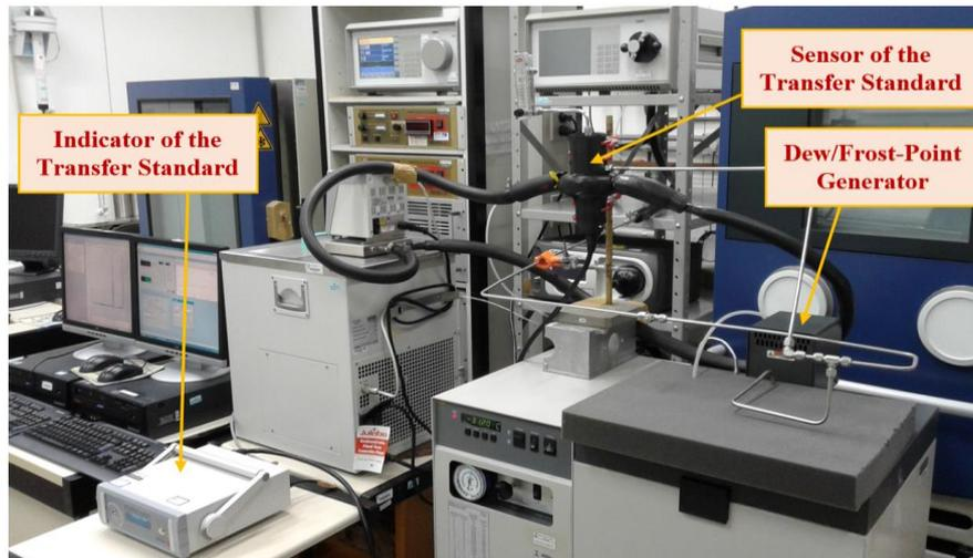
Figure 2 – Transfer Standard Sensor Connected at the Dew/Frost-Point Generator of INMETRO
