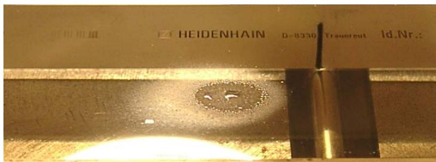
**Fig. 7:** Example of severe contamination of circulated standard.
