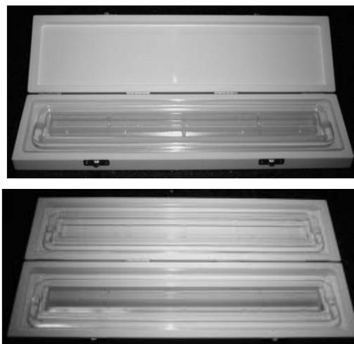
Fig. 6: Line scale box with Zerodur scale.
