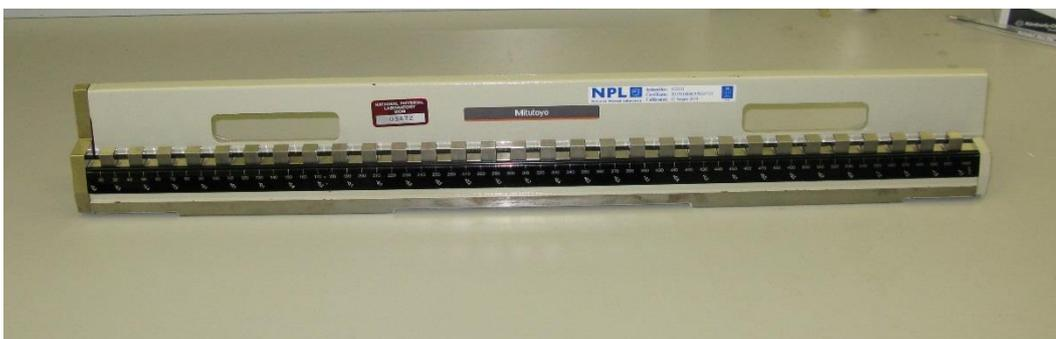
Figure 4: 610 mm step gauge
