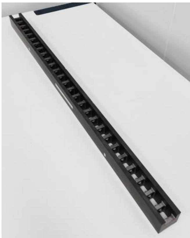
Figure 1: Ceramic 1020 mm step gauge
