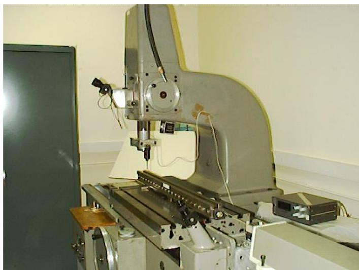
This machine has an X movement on which the axe of the step gauge is aligned and a vertical movement, in order to enter to the center line.
