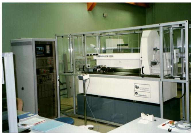
*Interferometric Comparator CEM-TEK 1200*
