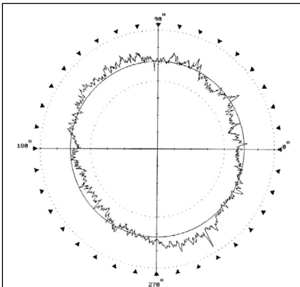
**Fig. C3.** 49.3 mm ring. Scale= 0.1 μm
