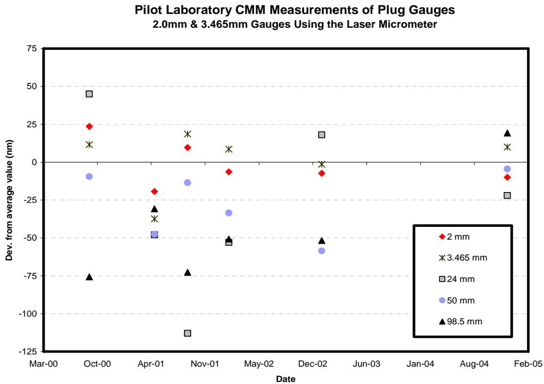
Figure 2. Pilot laboratory measurements of external diameter standards.
