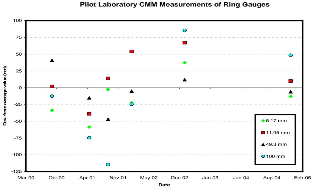
Figure 1. Pilot laboratory measurements of internal diameter standards.
