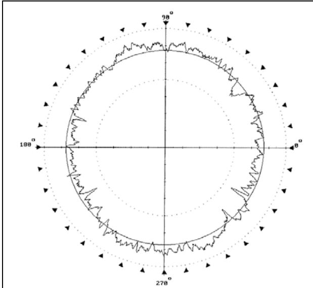
**Fig. C1.** 5.17 mm ring, Scale= 0.1 μm
