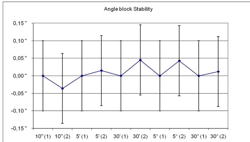
**Figure 2.** Stability of 5 angle blocks between the first LNE measurement (1: August 2014) and the second measurement (2: October 2014). In order to have all the values in the same range, the "0" value correspond to the deviation from nominal angle of the first measurements (1) for each angle block. Error bars correspond to the standard uncertainty ( $k=1$ ).
