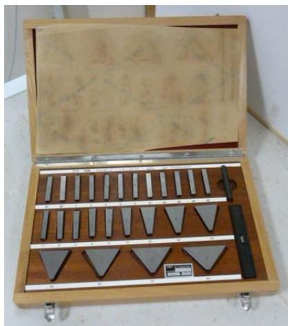
**Figure 1 :** Image of the angle block box. There are 25 angle blocks, only the 10", 5', 30', 5°, 30° angle blocks will be measured. The others should be kept untouched under grease protection.
