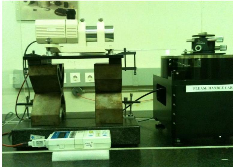
**Figure 5** :KIM-LIPI set up measurement of angle block
