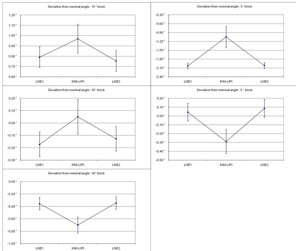
**Figure 3.** Results for deviation from nominal angle  $d$  in seconds (") for all of the angle blocks. Error bars: Standard uncertainty ( $k=1$ ).
