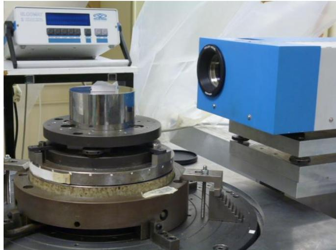
**Figure 4** : LNE set-up for angle block calibration
