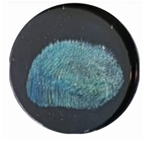
Figure 4: Face 4 of the 12-sided polygon with serial number 327. A large finger print dominates the mirror surface.
