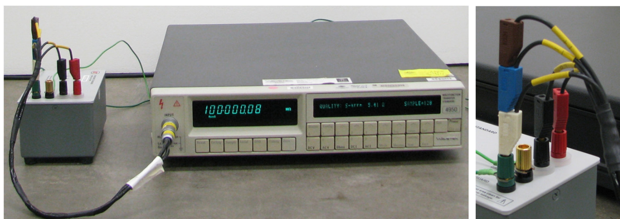
Figure VIII-5: Wiring diagram for two wire resistance measurements
