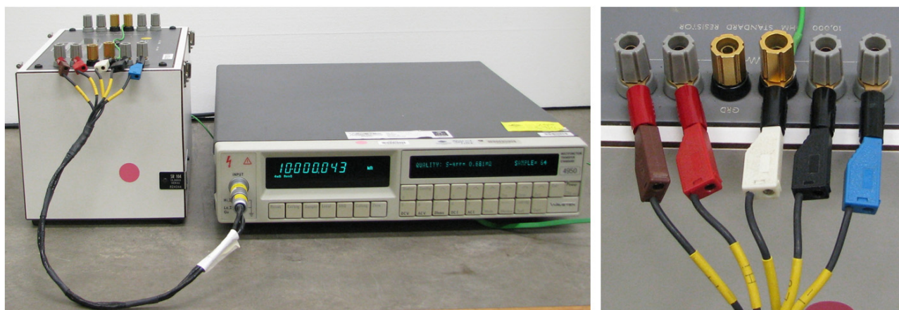
Figure VIII-4: Wiring diagram for four wire resistance measurements
