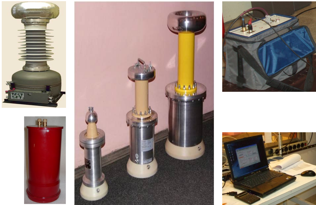
Picture 1 - VNIIMS reference measuring system (RMS)
