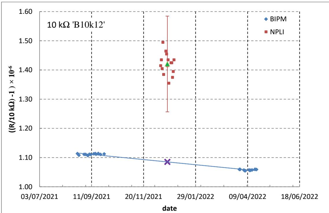
**Figure 5: Results for 10 kΩ standard B10K12. BIPM (blue diamonds) and NPLI (red squares) measurements. The cross corresponds to the extrapolated BIPM measurement at the mean date of measurement at NPLI and the green triangle is the mean value of NPLI measurements. The uncertainty bar shows the expanded uncertainty of the comparison of the mean NPLI results.**
