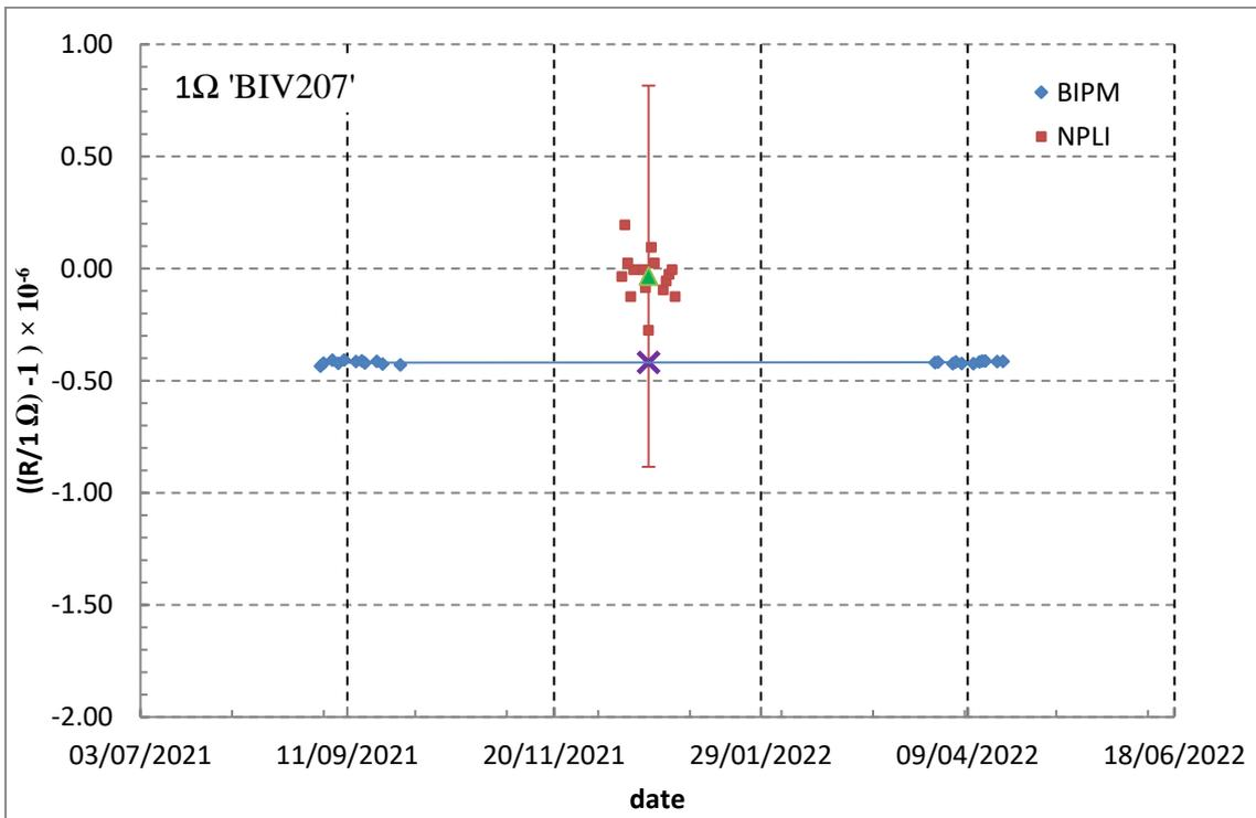
**Figure 3: Results for 1 Ω standard BIV207. BIPM (blue diamonds) and NPLI (red squares) measurements. The cross corresponds to the extrapolated BIPM measurement at the mean date of measurement at NPLI and the green triangle is the mean value of NPLI measurements. The uncertainty bar shows the expanded uncertainty of the comparison of the mean NPLI results.**
