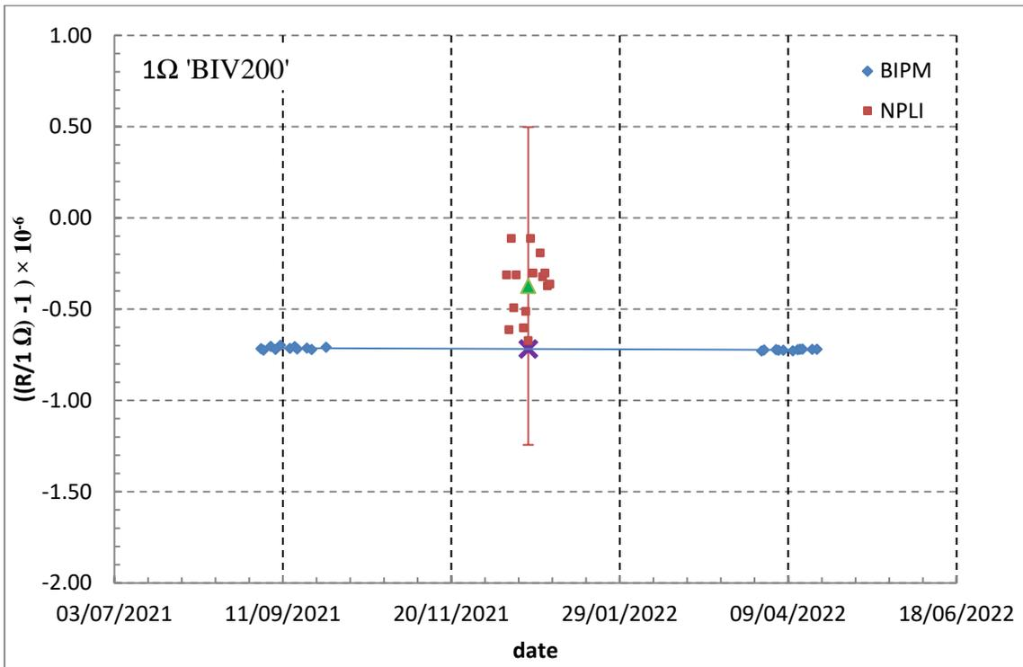
**Figure 2: Results for 1 Ω standard BIV200. BIPM (blue diamonds) and NPLI (red squares) measurements. The cross corresponds to the extrapolated BIPM measurement at the mean date of measurement at NPLI and the green triangle is the mean value of NPLI measurements. The uncertainty bar shows the expanded uncertainty of the comparison of the mean NPLI results.**
