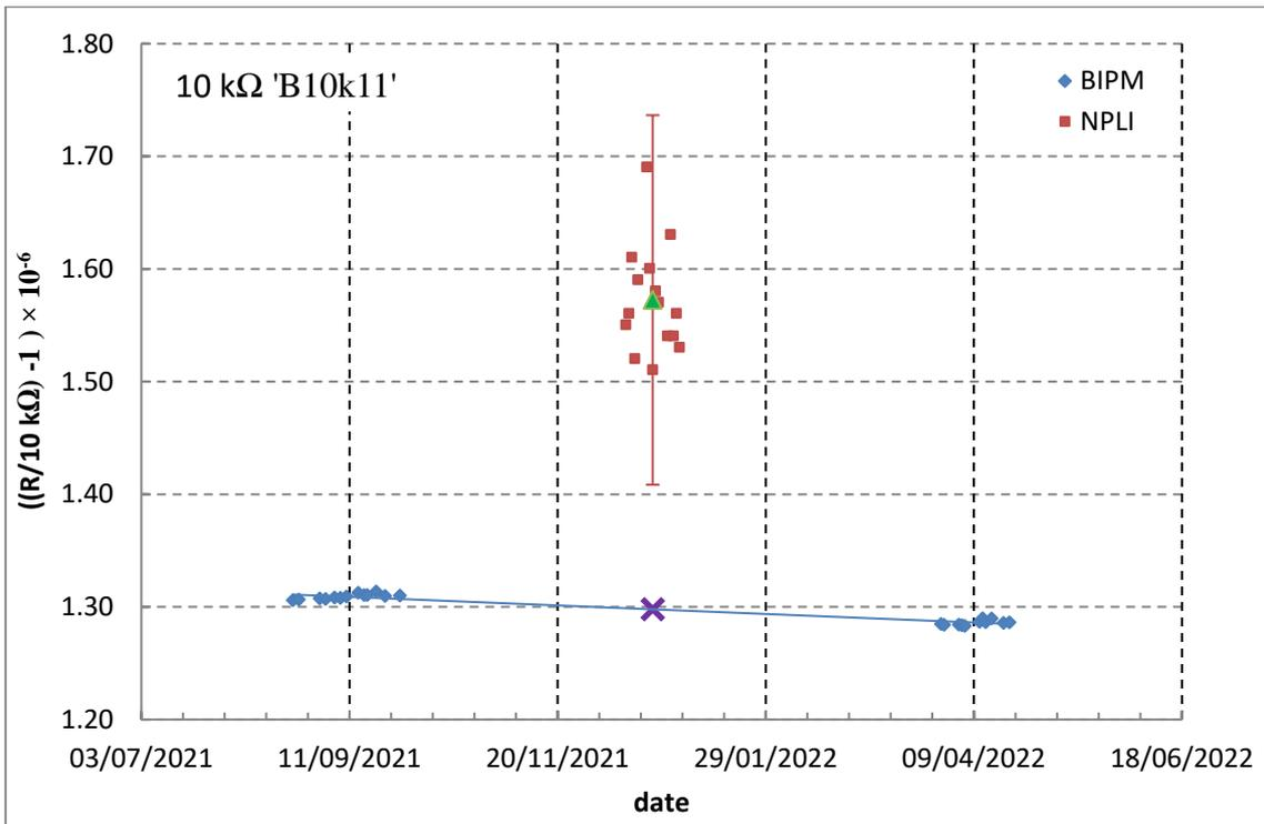
**Figure 4: Results for 10 kΩ standard B10K11. BIPM (blue diamonds) and NPLI (red squares) measurements. The cross corresponds to the extrapolated BIPM measurement at the mean date of measurement at NPLI and the green triangle is the mean value of NPLI measurements. The uncertainty bar shows the expanded uncertainty of the comparison of the mean NPLI results.**
