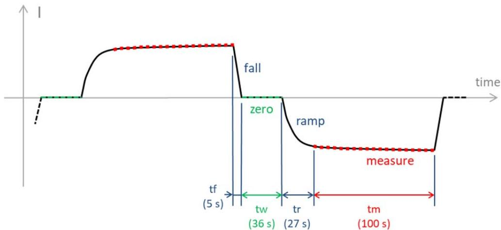
**Figure 1: Schematic representation of the reference current signal with polarity reversals used in the BIPM CCC-bridge. The reversal cycle comprises a waiting time of about 36 s at zero current (green dotted line). The red dotted line corresponds to the sampling time period.**
