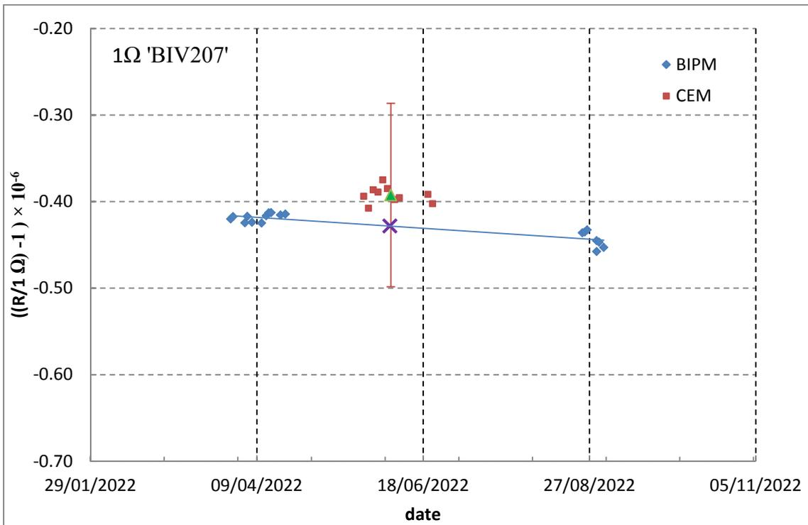
**Figure 4: Results for 1 Ω standard BIV207. BIPM (blue diamonds) and CEM (red squares) measurements. The cross corresponds to the extrapolated BIPM measurement at the mean date of measurement at CEM and the green triangle is the mean value of CEM measurements. The uncertainty bar shows the expanded uncertainty of the comparison of the mean CEM results.**
