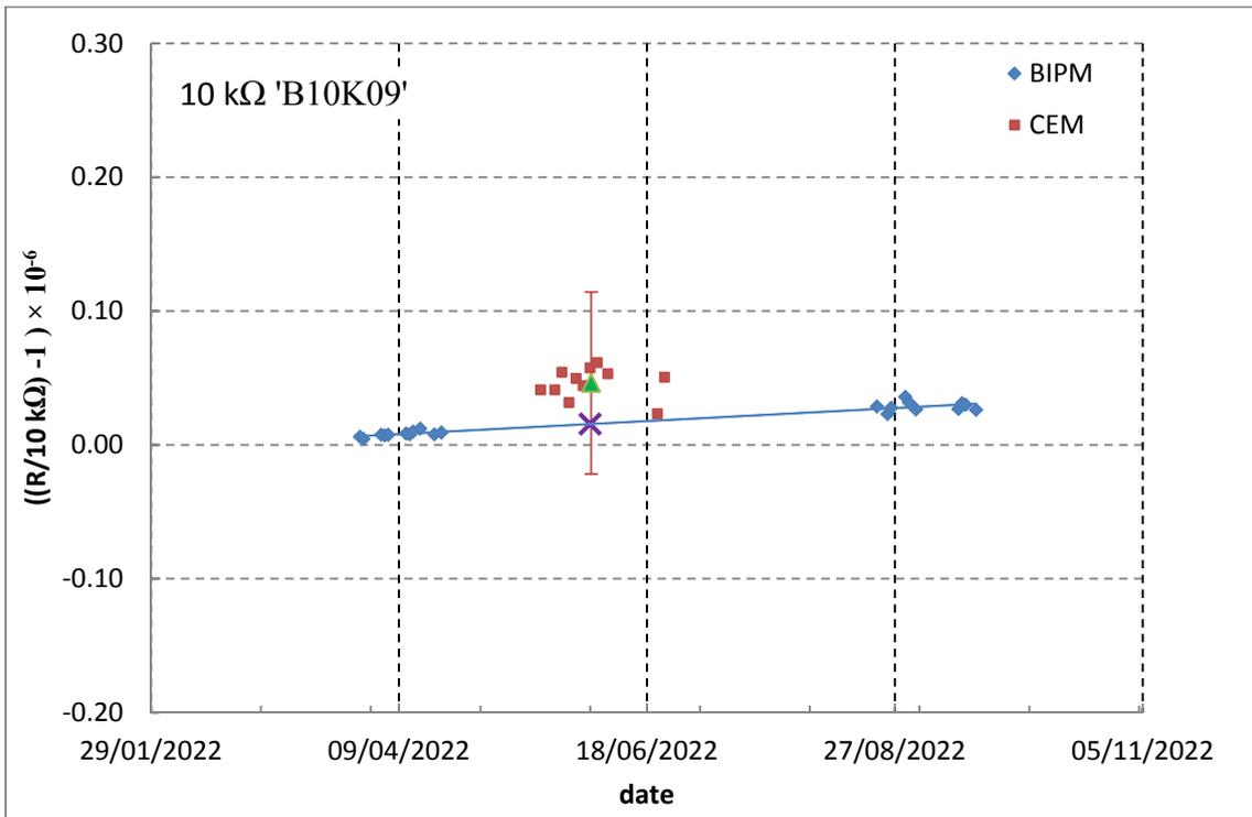
**Figure 5: Results for 10 kΩ standard B10K09. BIPM (blue diamonds) and CEM (red squares) measurements. The cross corresponds to the extrapolated BIPM measurement at the mean date of measurement at CEM and the green triangle is the mean value of CEM measurements. The uncertainty bar shows the expanded uncertainty of the comparison of the mean CEM results.**
