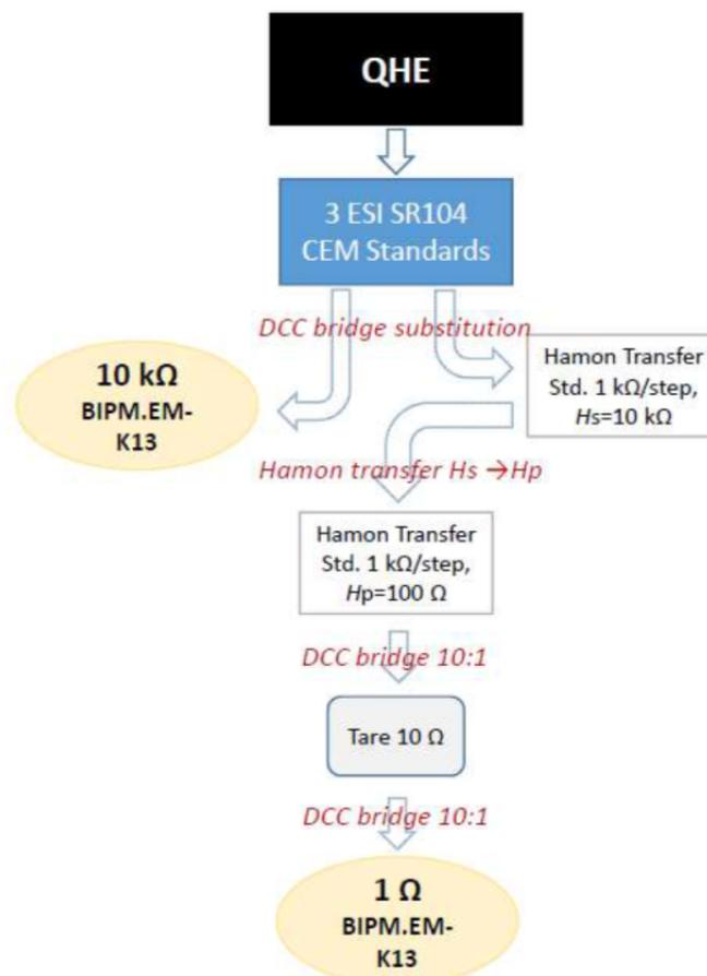
**Figure 2: Schematic representation of the traceability chain for the calibration of the comparison standards at the CEM.**
