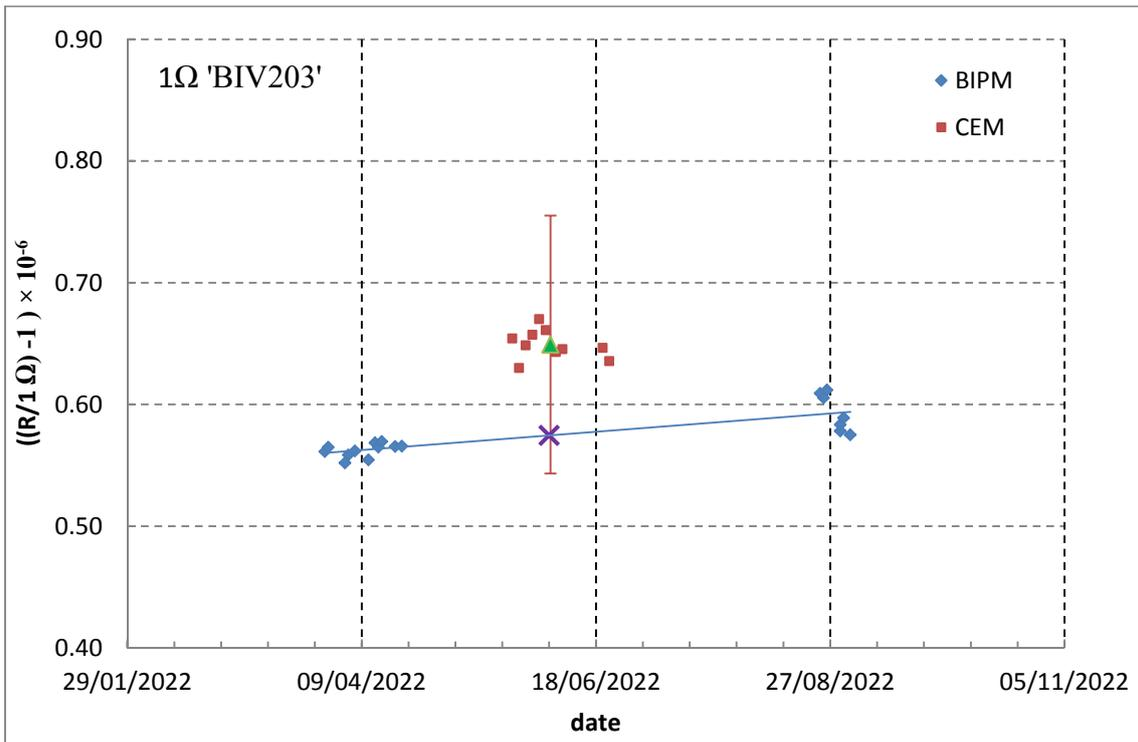
**Figure 3: Results for 1 Ω standard BIV203. BIPM (blue diamonds) and CEM (red squares) measurements. The cross corresponds to the extrapolated BIPM measurement at the mean date of measurement at CEM and the green triangle is the mean value of CEM measurements. The uncertainty bar shows the expanded uncertainty of the comparison of the mean CEM results.**
