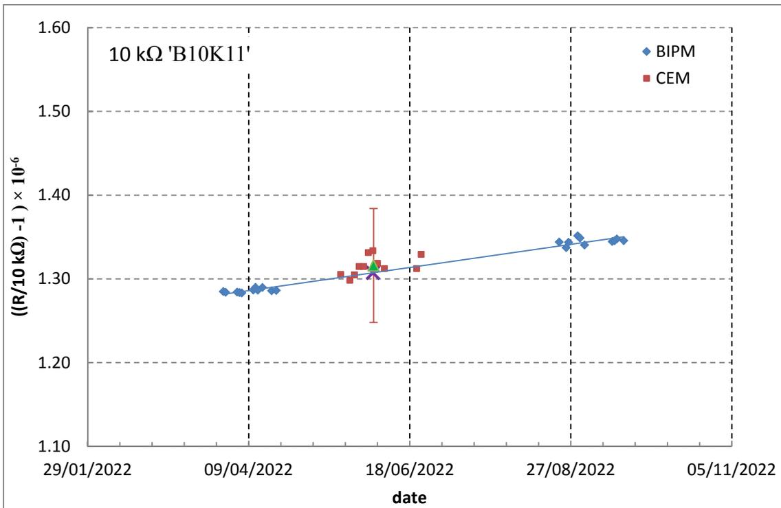
**Figure 6: Results for 10 kΩ standard B10K11. BIPM (blue diamonds) and CEM (red squares) measurements. The cross corresponds to the extrapolated BIPM measurement at the mean date of measurement at CEM and the green triangle is the mean value of CEM measurements. The uncertainty bar shows the expanded uncertainty of the comparison of the mean CEM results.**
