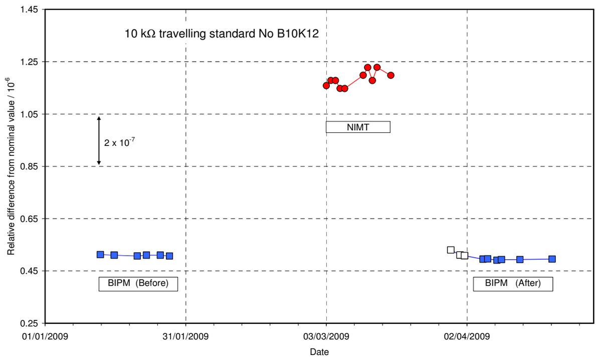
Figure 2: Calibrations at the BIPM (squares) and at the NIMT (circles) of the travelling standard ref. B10K12, expressed as the relative deviation from the nominal 10 kΩ value. The white squares correspond to transient values not used in the calculation.
