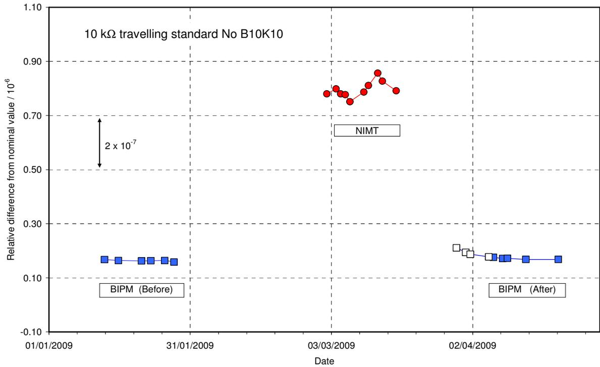
Figure 1: Calibrations at the BIPM (squares) and at the NIMT (circles) of the travelling standard ref. B10K10, expressed as the relative deviation from the nominal 10 kΩ value. The white squares correspond to transient values not used in the calculation.
