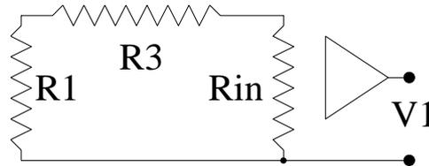
Figure 7: Equivalent circuit for determining AC/DC transfer standard input impedance
