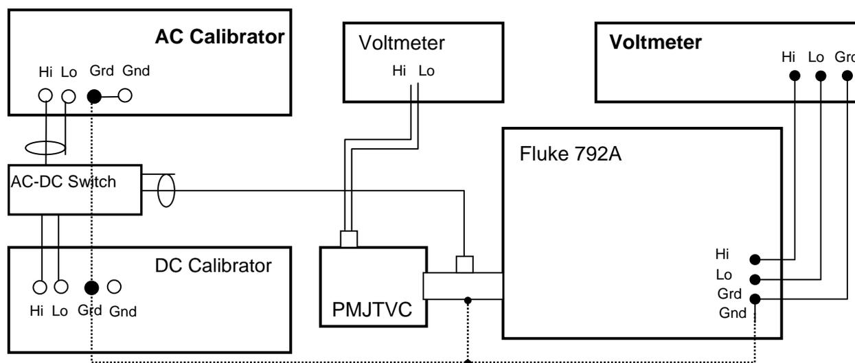
**Figure 1.** Measurement set-up for 100 mV measurements
