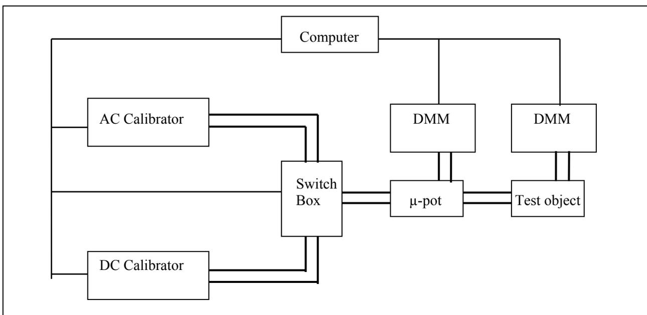
Fig. 2: Step-down set-up using  $\mu$ -pots.
