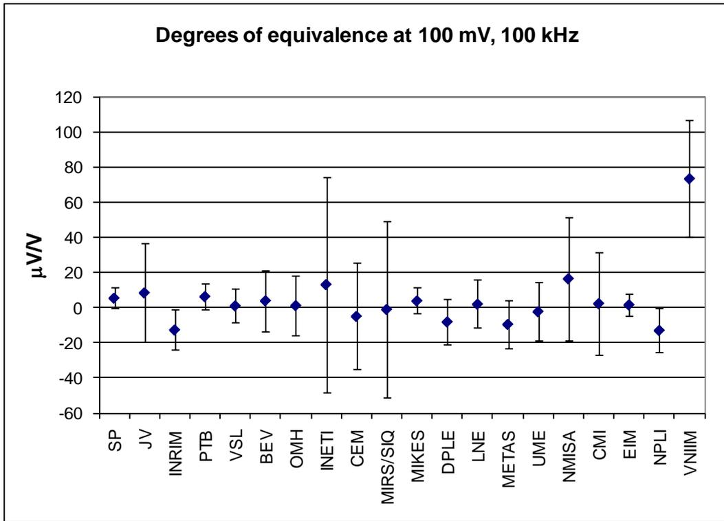
Figure 13 Degree of equivalence with the CRV at 100 mV, 100 kHz with corresponding expanded uncertainties ( $k=2$ ).
