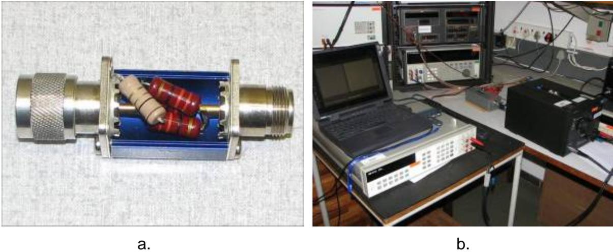
Figure 4: a. Resistive divider detail, and b. Setup to determine input impedance.
