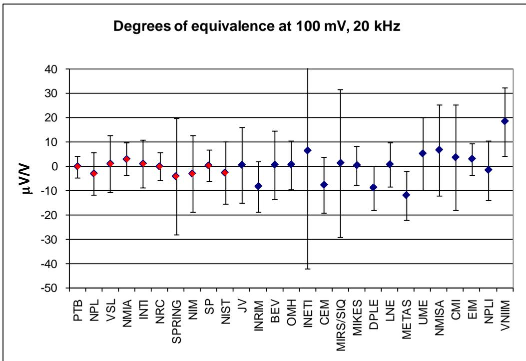
Figure 21 Degree of equivalence with the KCRV at 100 mV, 20 kHz with corresponding expanded uncertainties ( $k=2$ ).
