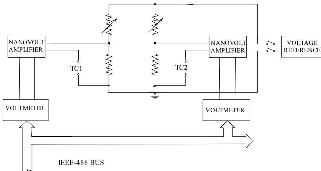
**Fig. 3** Basic circuit of the EMFs comparator.
