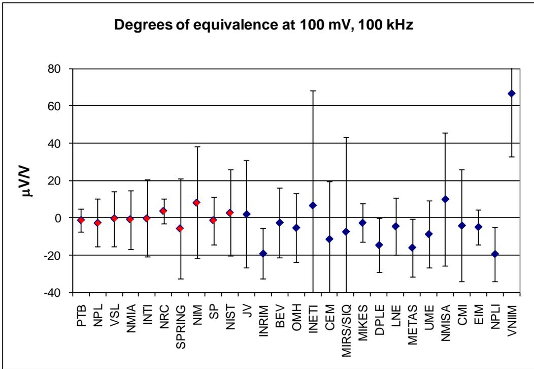
Figure 22 Degree of equivalence with the KCRV at 100 mV, 100 kHz with corresponding expanded uncertainties (k=2).
