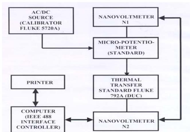
*Fig. 1: Block Diagram Of Low Voltage Inter-Comparison For Measurement Of AC-DC Transfer Difference*
