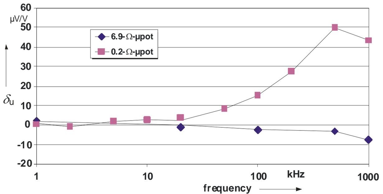
Fig. 3 Ac-dc voltage transfer difference  $\delta$  of the 6.9- $\Omega$ - $\mu$ pot and the 0.2- $\Omega$ - $\mu$ pot at 100 mV.
