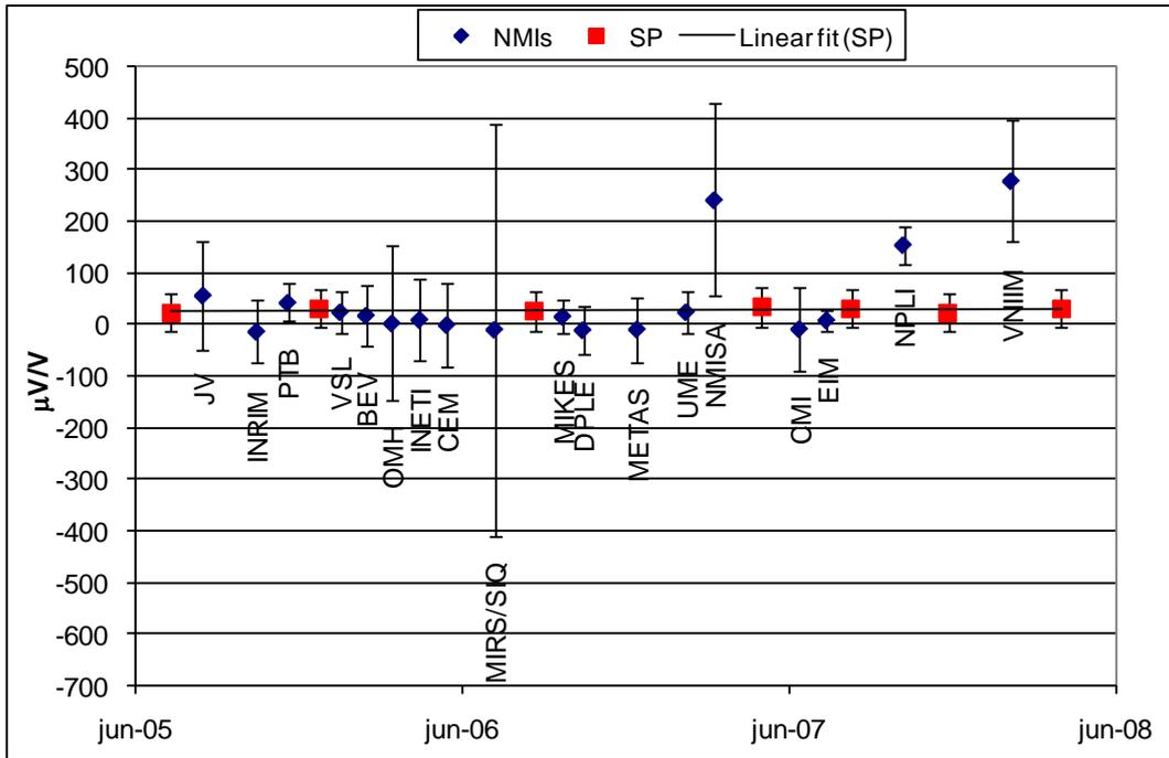
Figure 4 Reported values  $\delta_i$ , 100 mV, 1 MHz, and stability of travelling standard
