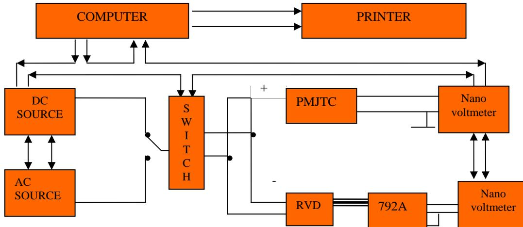
**Fig. 1. ac/dc transfer system. CEM**
