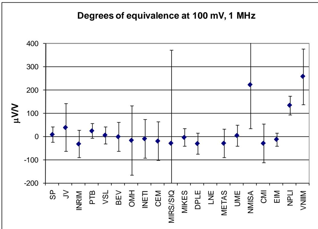
Figure 14 Degree of equivalence with the CRV at 100 mV, 1 MHz with corresponding expanded uncertainties ( $k=2$ ).
