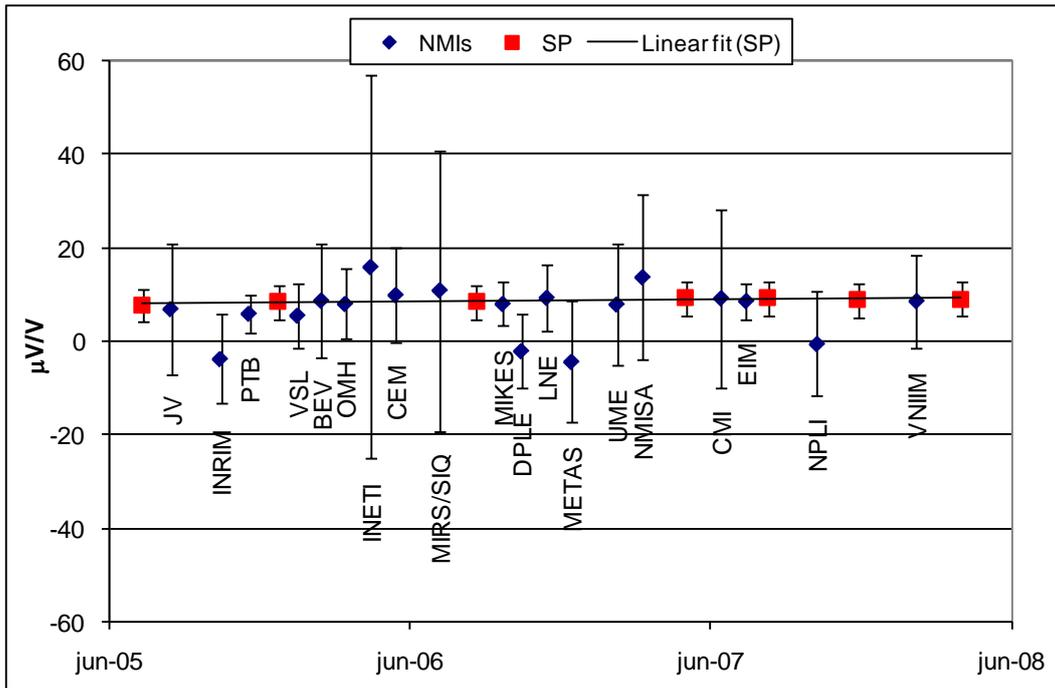
Figure 1 Reported values  $\delta_i$ , 100 mV, 1 kHz, and stability of travelling standard
