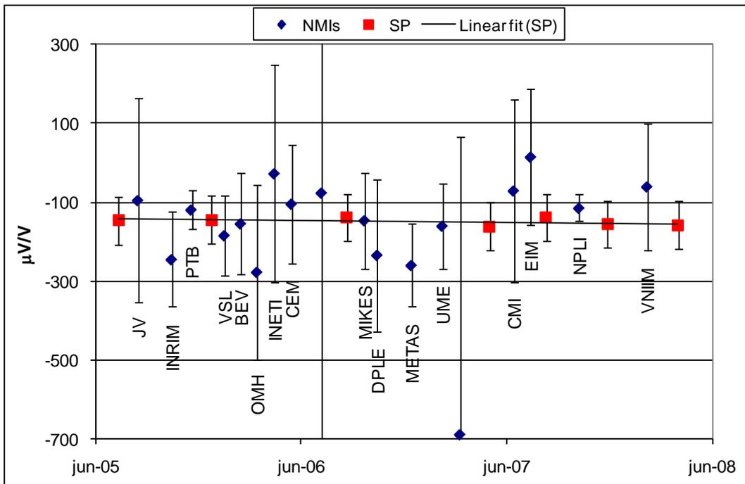
Figure 10 Reported values  $\delta_i$ , 10 mV, 1 MHz, at larger scale, and stability of travelling standard
