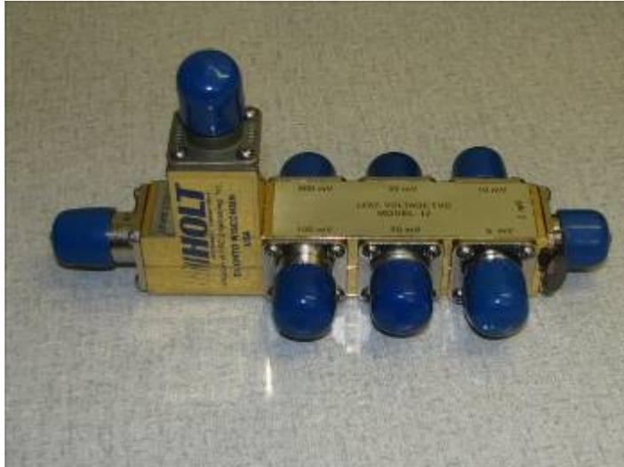
Figure 1: Holt model 12 low-voltage thermal transfer standard (LVTVC).
