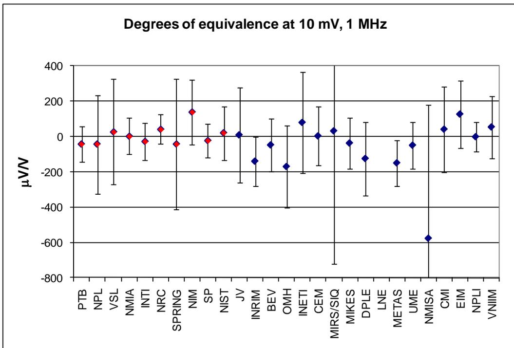
Figure 27 Degree of equivalence with the KCRV at 10 mV, 1 MHz with corresponding expanded uncertainties (k=2).
