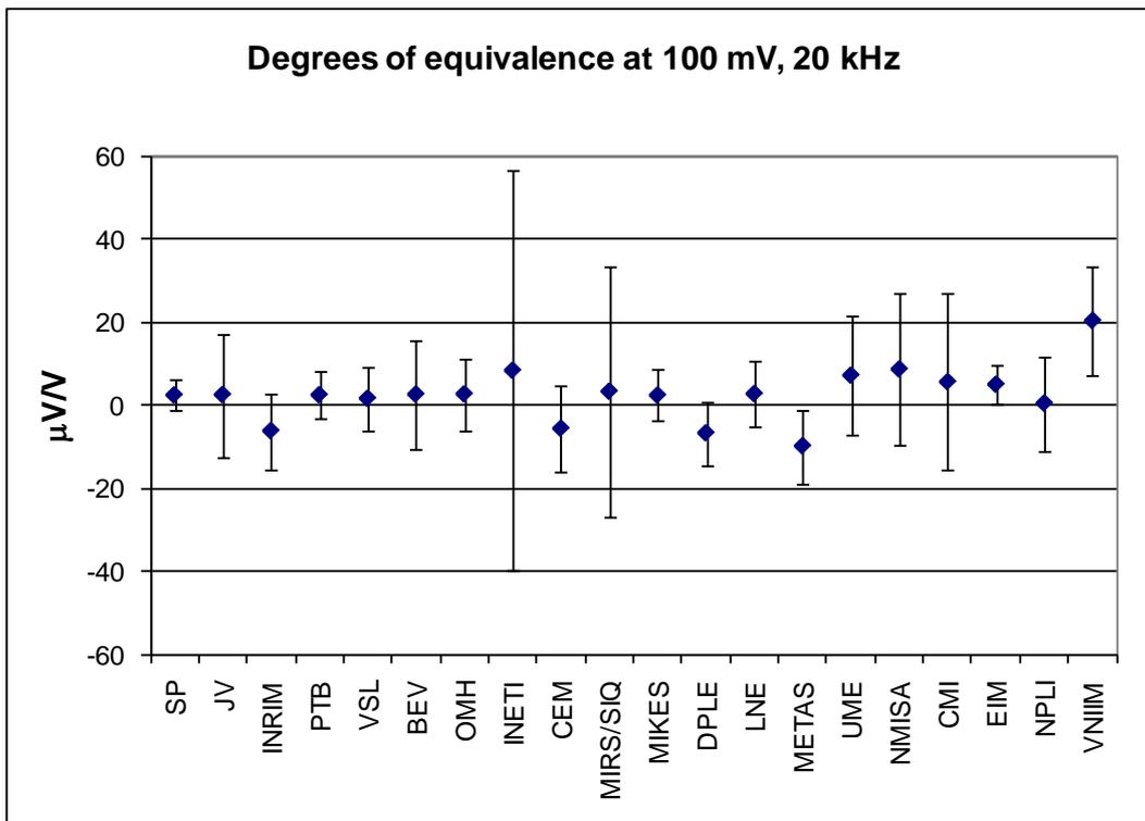
Figure 12 Degree of equivalence with the CRV at 100 mV, 20 kHz with corresponding expanded uncertainties (k=2).
