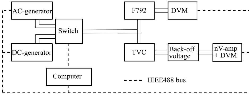
Fig. 1. Automated measuring system for comparison of Fluke 792A and PMJTC.
