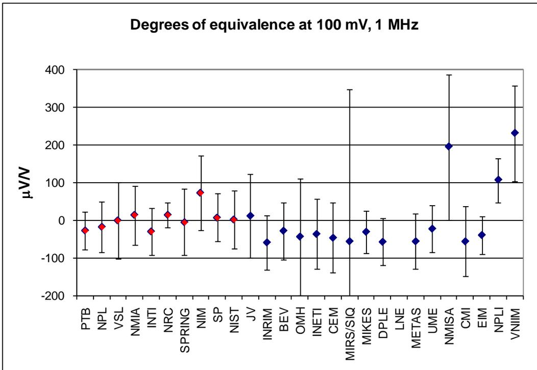
Figure 23 Degree of equivalence with the KCRV at 100 mV, 1 MHz with corresponding expanded uncertainties (k=2).
