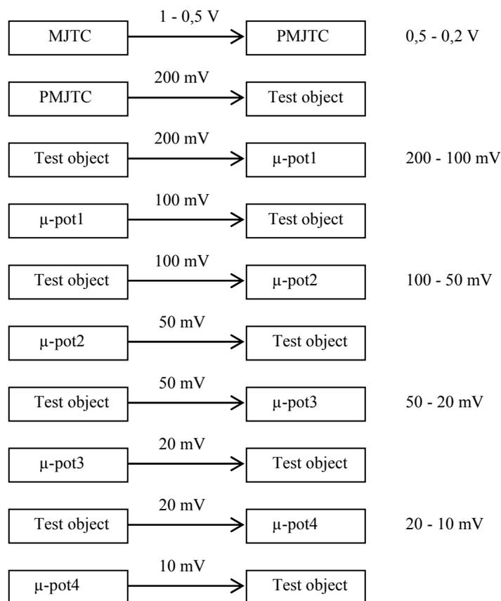
Fig. 3: Step-down procedure.
