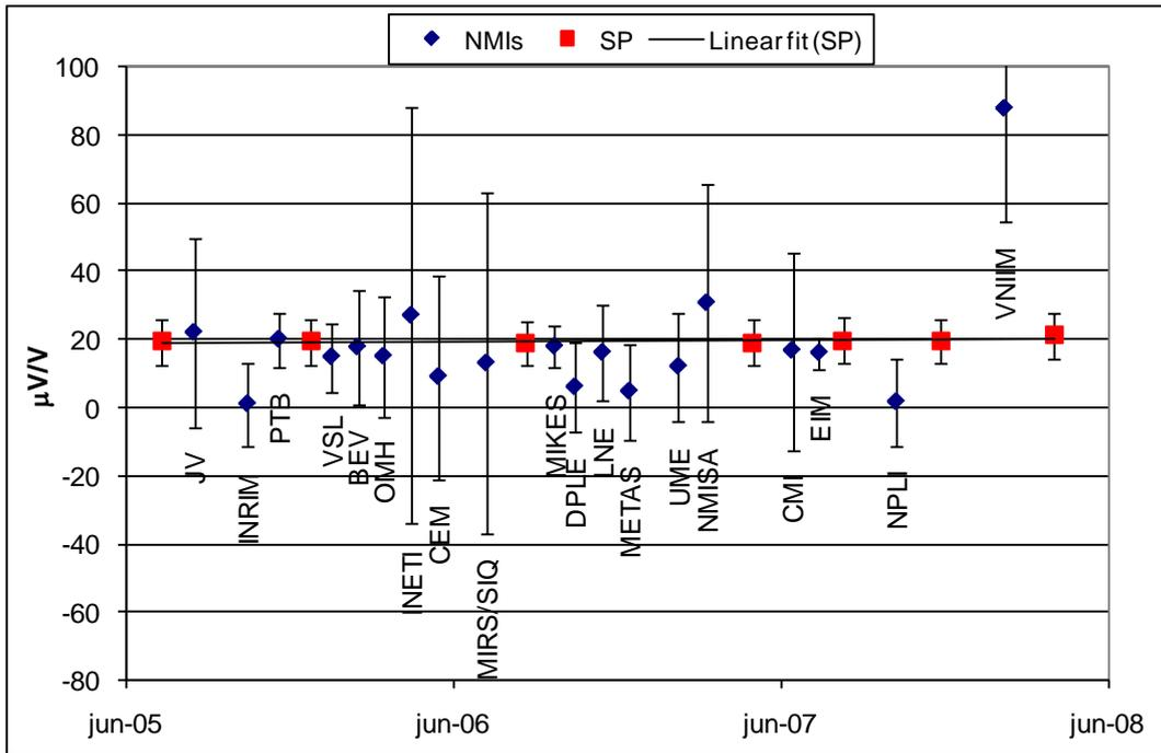
Figure 3 Reported values  $\delta_i$ , 100 mV, 100 kHz, and stability of travelling standard
