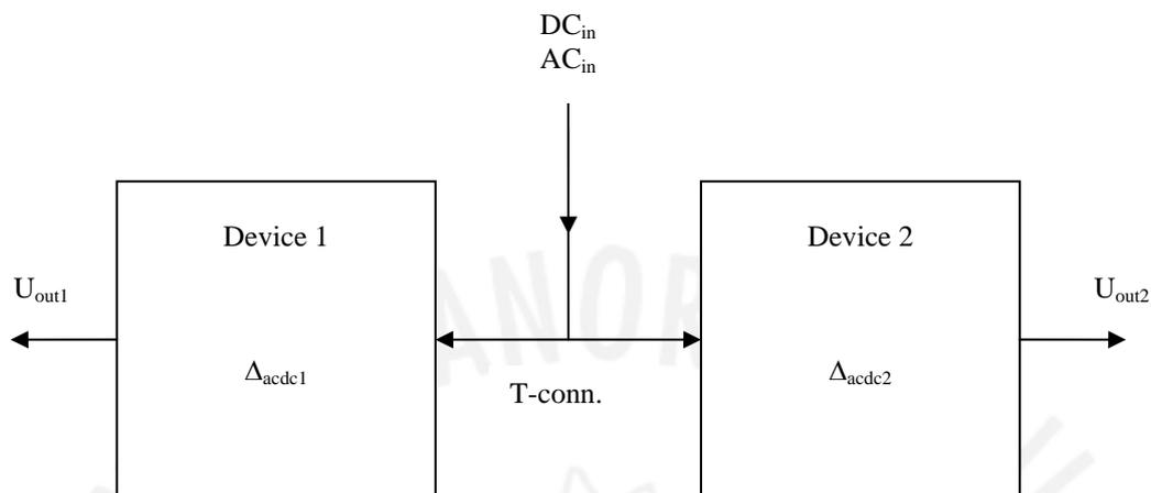
Input voltages are  $DC_{in}$  and  $AC_{in}$ .  $AC_{in}$  is the RMS value of AC voltage.
