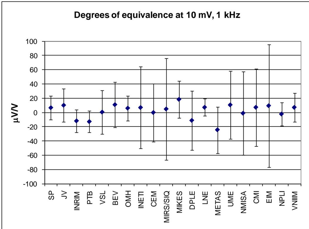
Figure 15 Degree of equivalence with the CRV at 10 mV, 1 kHz with corresponding expanded uncertainties (k=2).
