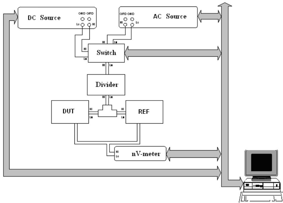
**Fig. 2** Measurement system for 100mV
