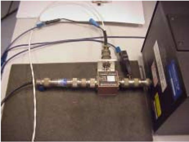
Figure 4 shows the set-up of the measurements between the Ballantine 1351 en de SP\_Fluke 792A. A special N-male to N-male is used to connect the central ground. Also the low output of the thermal element of the micropotentiometer is connected to the central ground.
