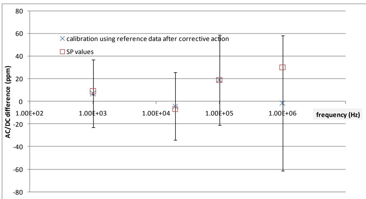
Figure 2: calibration of travelling standard at 100 mV: comparison of the values obtained by SP (squares) and of the METAS measurement during EM-K11 done with own's 792 A (crosses). The calibration values of METAS' own instrument are those obtained in 2010. Error bars correspond to METAS uncertainty (k=2)
