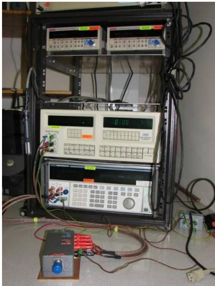
Figure 2: CSIR NML ac-dc difference measurement setup.
