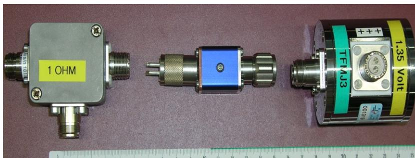
Figure 1: view of a micropotentiometer of inappropriate construction. Left: housing for the disk resistor, middle: adapter, right: planar multijunction converter in brass housing.
