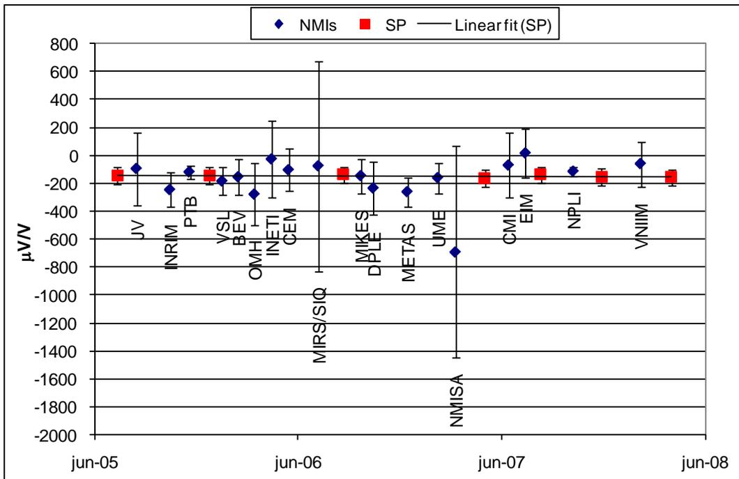
Figure 9 Reported values  $\delta_{ic}$ , 10 mV, 1 MHz, and stability of travelling standard
