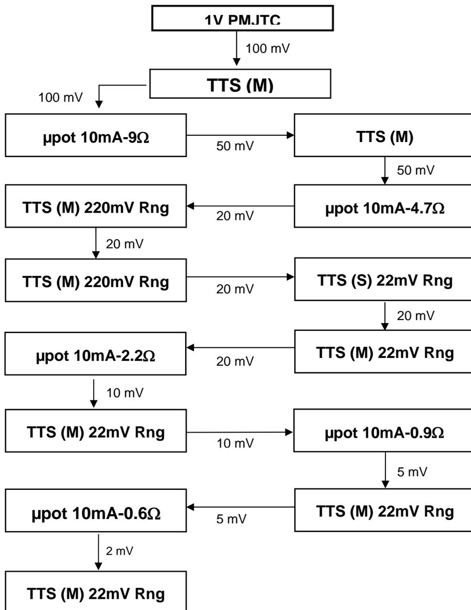
TVC, which is used to calibrate 100 mV voltage of TTS is a 1V planar multi-junction TVC calibrated by PTB as part of a group of several converters in range of 1V-3 V. This group forms primary basis of the step-up and step-down procedures in UME.  $\mu$ POTs used in calibration are combination of the Ballantine 1251 model thermal housing and 1351 model disk resistors. Values and usable voltage ranges of all combinations available at UME are shown in table:
