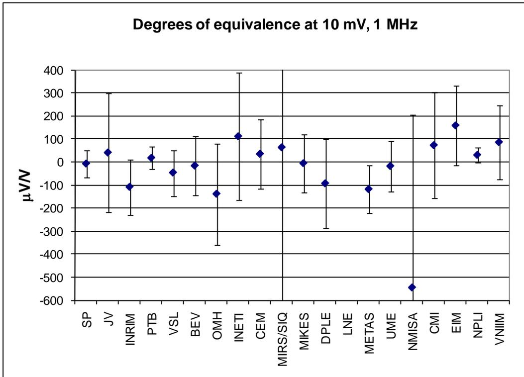
Figure 19 Degree of equivalence with the CRV at 10 mV, 1 MHz with corresponding expanded uncertainties ( $k=2$ ) at larger scale.
