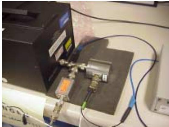
Figure 1. PMJTC-2 against SP 792A at 220 mV-range
