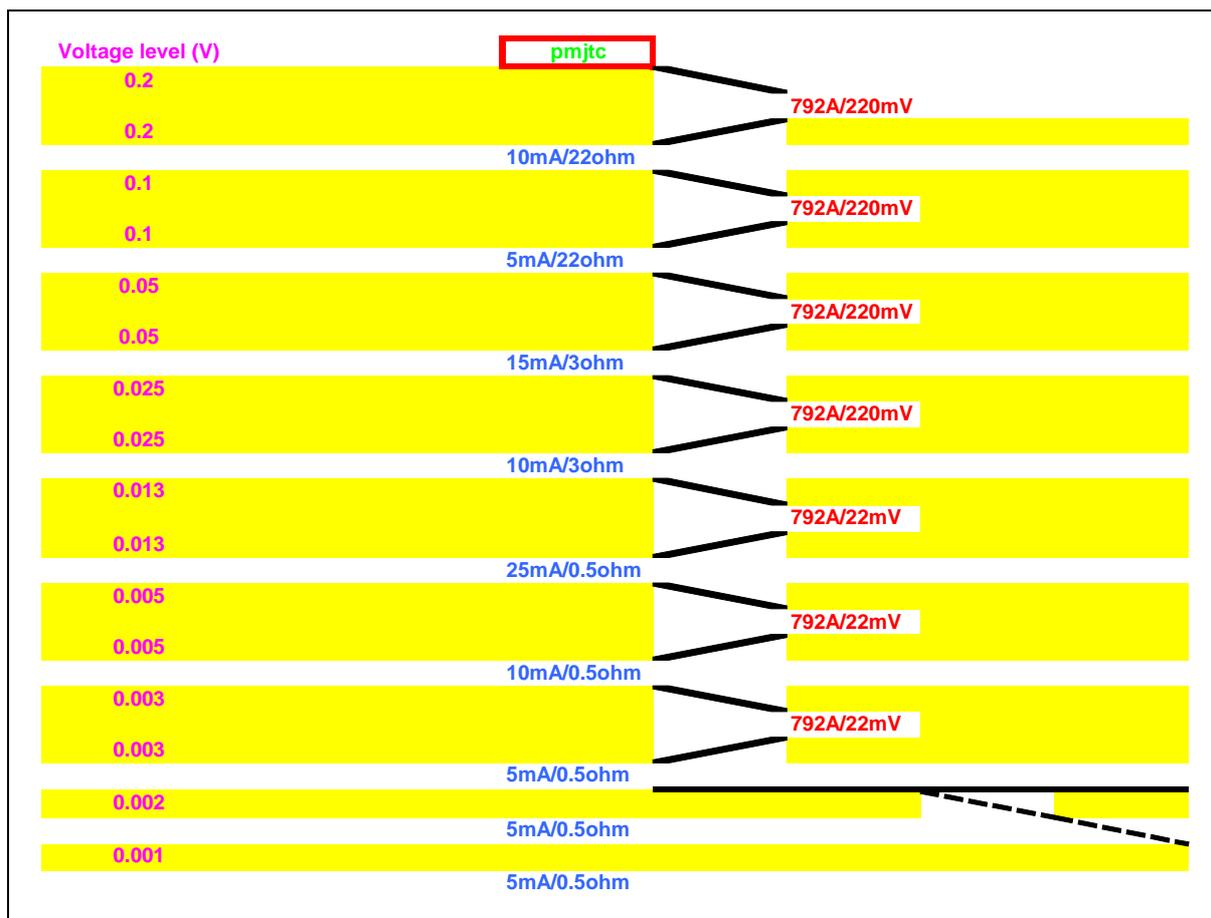
Figure 1 Schematic of the step-down procedure with micropotentiometers (method 1).
