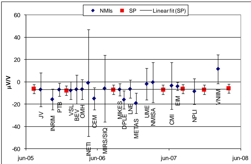
Figure 2 Reported values  $\delta_i$ , 100 mV, 20 kHz, and stability of travelling standard
