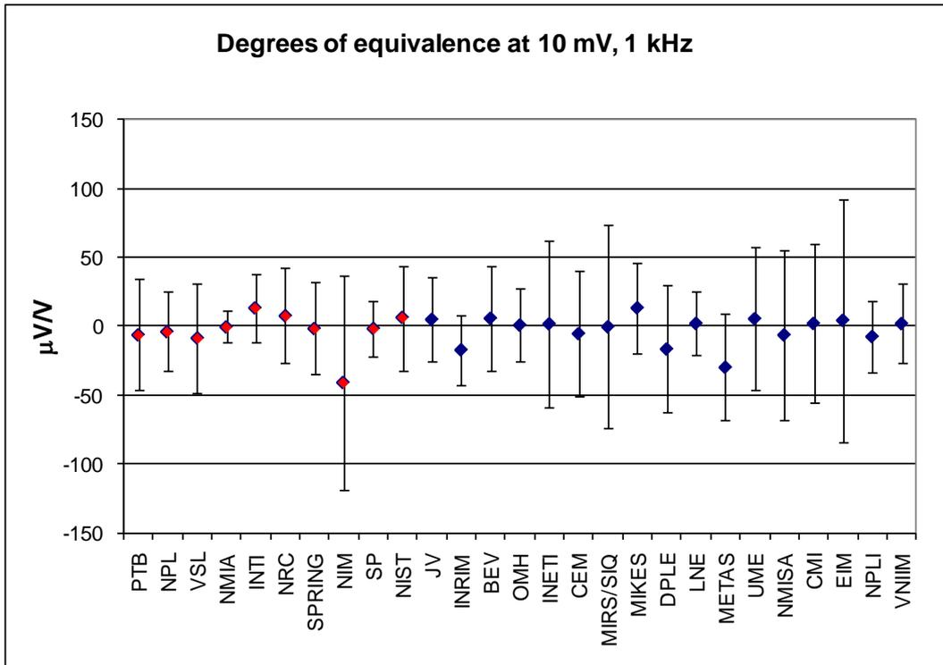
Figure 24 Degree of equivalence with the KCRV at 10 mV, 1 kHz with corresponding expanded uncertainties (k=2).
