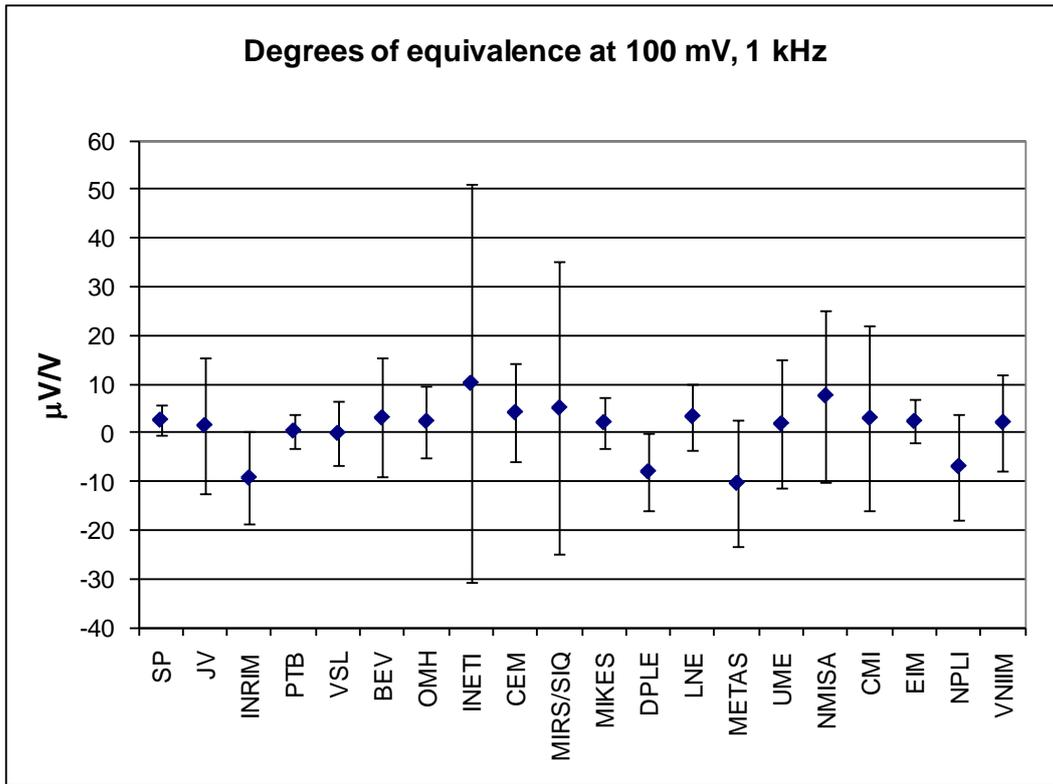
Figure 11 Degree of equivalence with the CRV at 100 mV, 1 kHz with corresponding expanded uncertainties (k=2).
