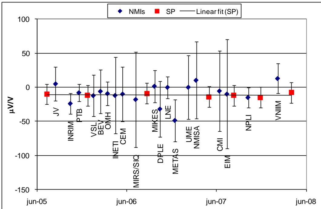
Figure 7 Reported values  $\delta_i$ , 10 mV, 20 kHz, and stability of travelling standard
