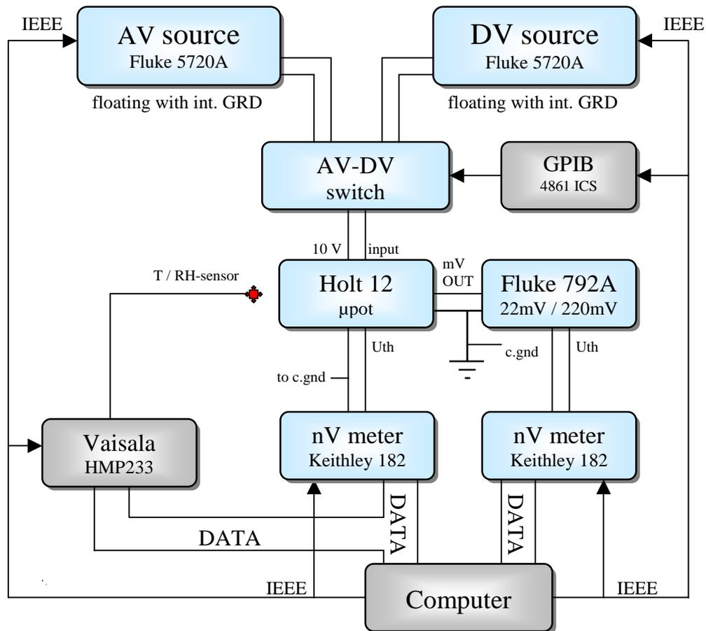
Figure 6. Measurement set-up realised on VSL operating system OS 4.
