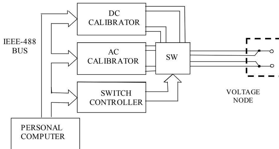
**Fig. 1** Basic circuit of the voltage generating system.
