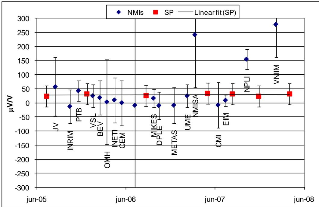
Figure 5 Reported values  $\delta_i$ , 100 mV, 1MHz, at lager scale, and stability of travelling standard
