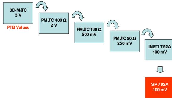
**Figure2: INETI's AC-DC Comparator**
