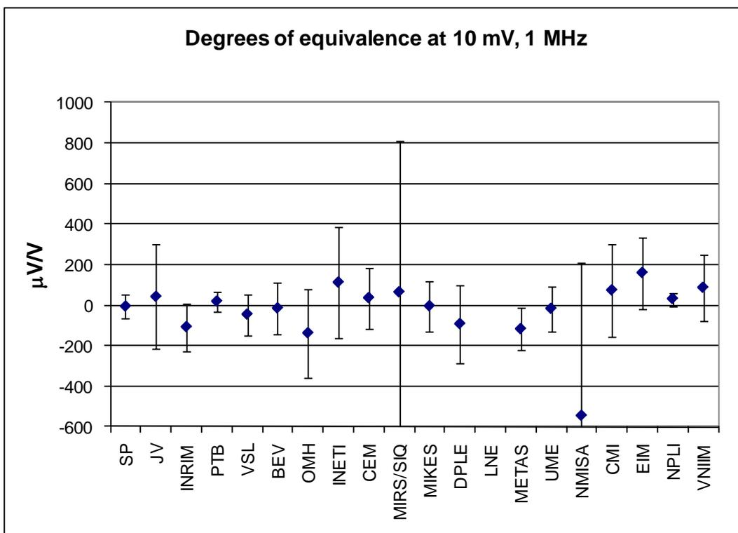
Figure 18 Degree of equivalence with the CRV at 10 mV, 1 MHz with corresponding expanded uncertainties ( $k=2$ ).
