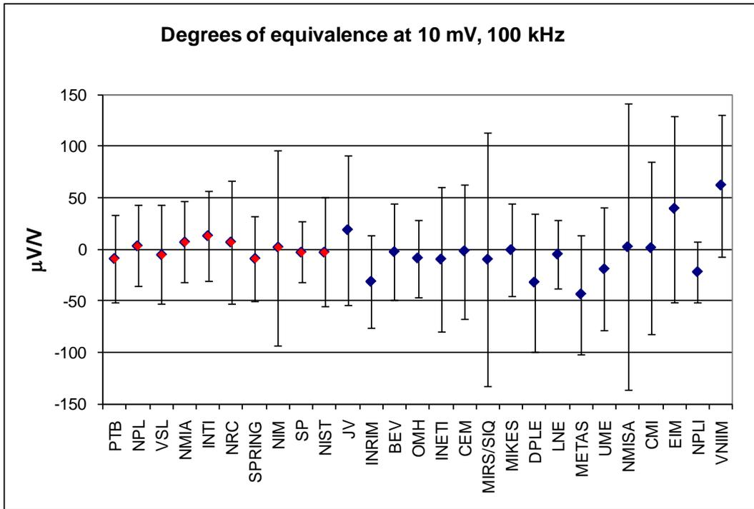
Figure 26 Degree of equivalence with the KCRV at 10 mV, 100 kHz with corresponding expanded uncertainties (k=2).
