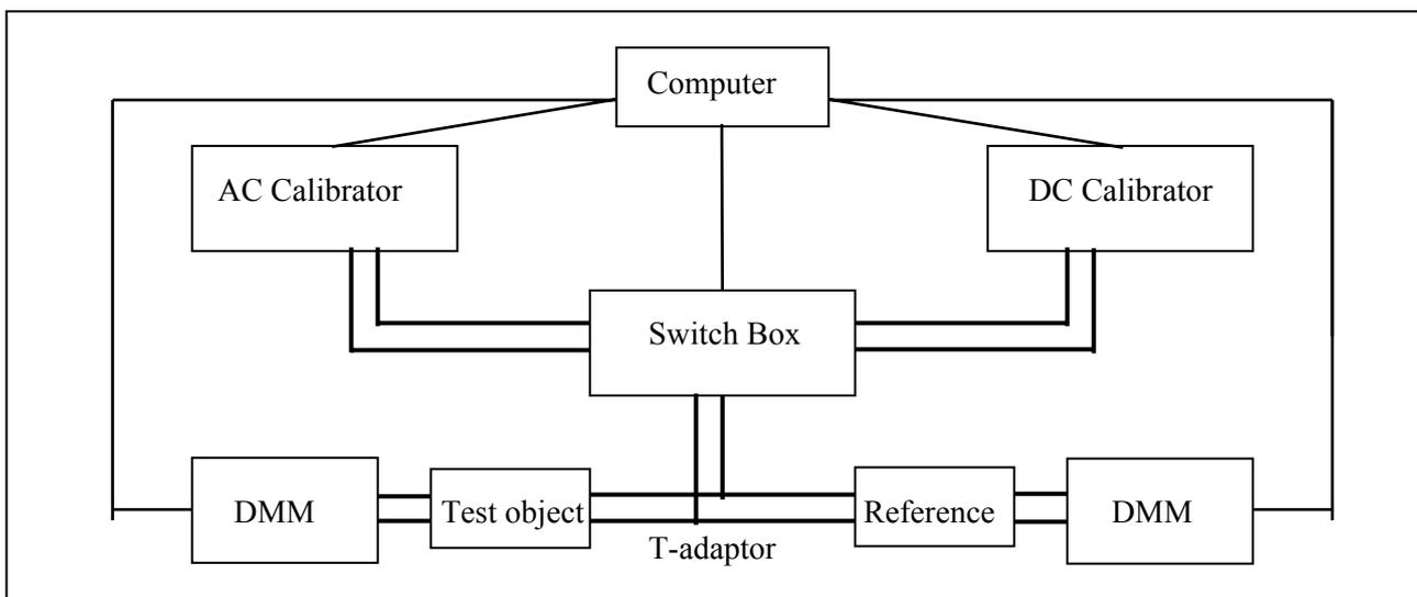
Fig. 1: Measurement set-up for the measurement of the AC-DC transfer difference of a thermal transfer standard.
