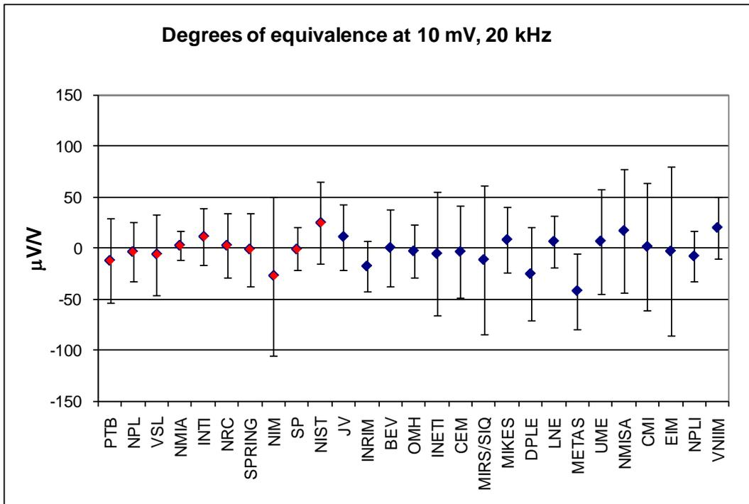
Figure 25 Degree of equivalence with the KCRV at 10 mV, 20 kHz with corresponding expanded uncertainties (k=2).
