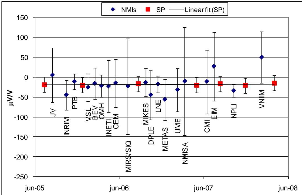
Figure 8 Reported values  $\delta_i$ , 10 mV, 100 kHz, and stability of travelling standard
