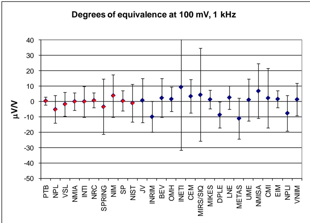
Figure 20 Degree of equivalence with the KCRV at 100 mV, 1 kHz with corresponding expanded uncertainties ( $k=2$ ).
