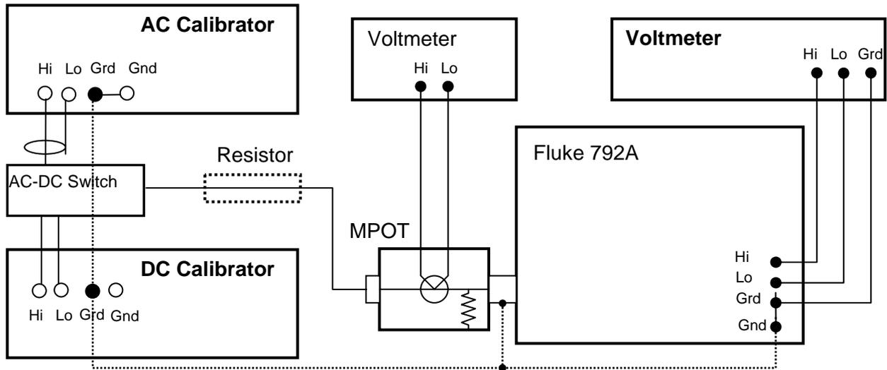
**Figure 2.** Measurement set-up for 10 mV measurements
