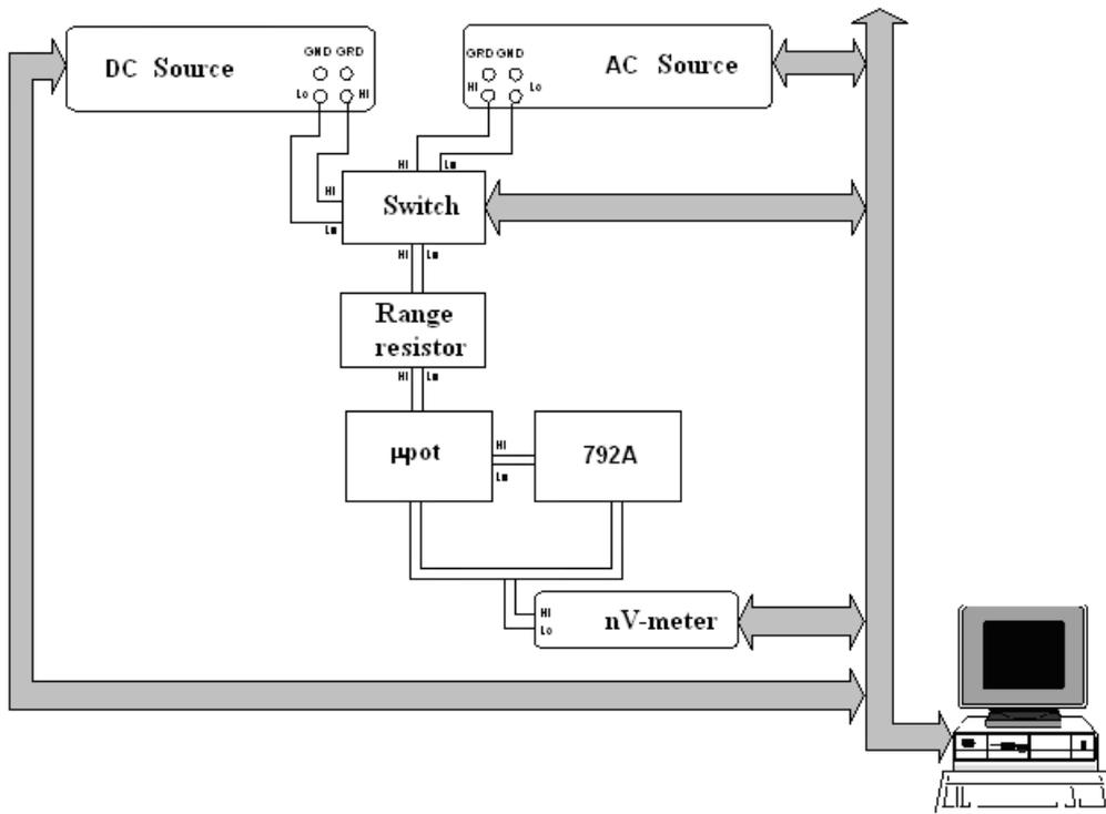
**Fig. 3** Measurement system below 100mV
