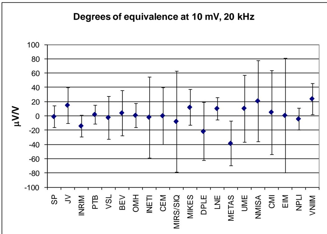
Figure 16 Degree of equivalence with the CRV at 10 mV, 20 kHz with corresponding expanded uncertainties (k=2).
