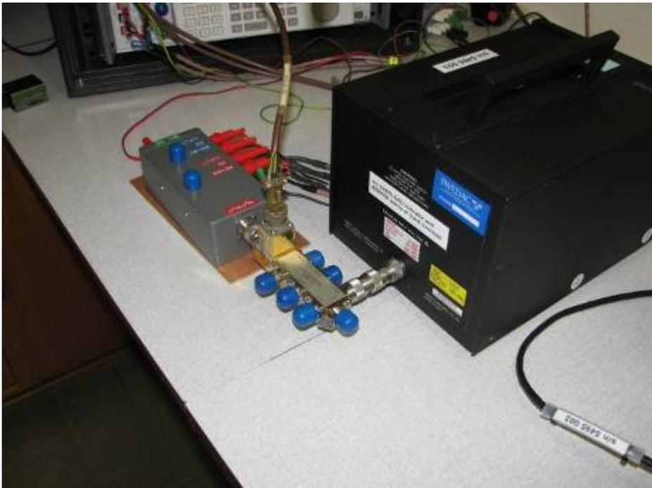
Figure 5: ac-dc difference measurement setup (for 10 mV measurement).
