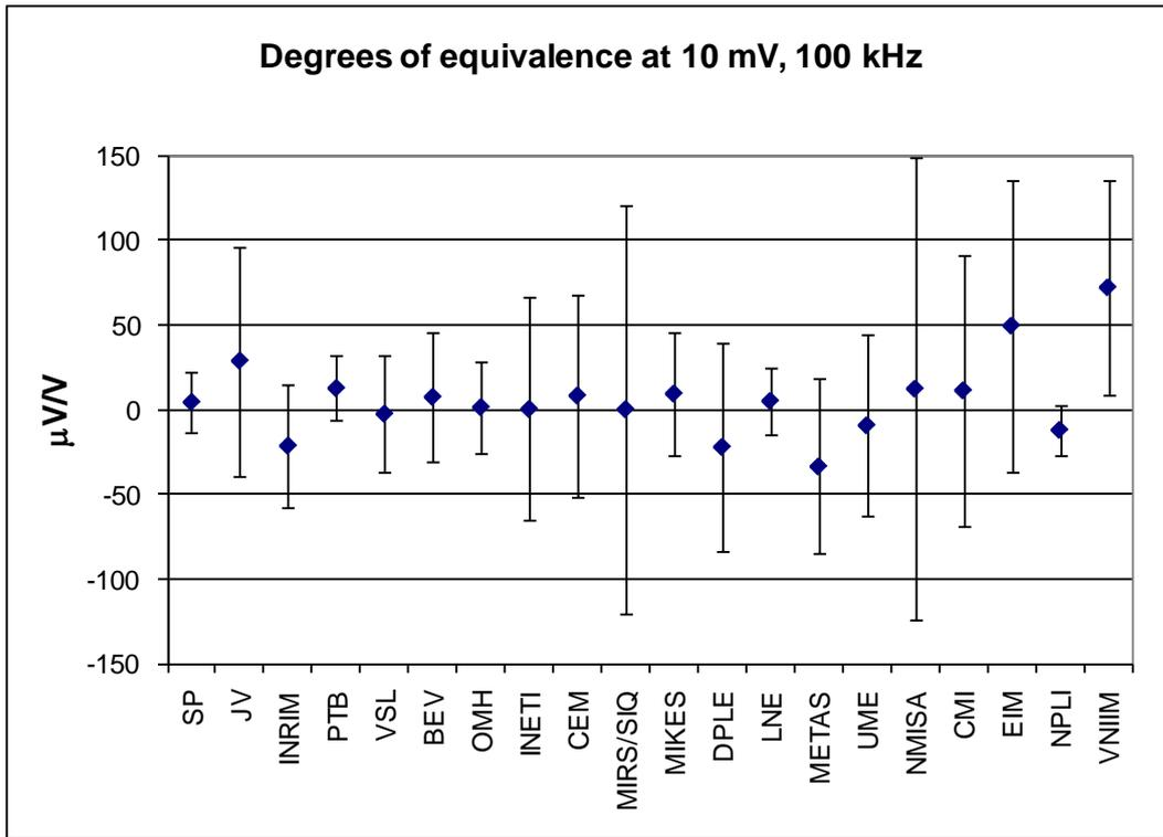
Figure 17 Degree of equivalence with the CRV at 10 mV, 100 kHz with corresponding expanded uncertainties ( $k=2$ ).
