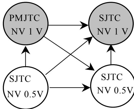
**Fig.4** Example of the measurement in the step-down procedure at 0.5 V. Four standards of different nominal voltage (two already calibrated in the previous step) are compared at 0.5 V
