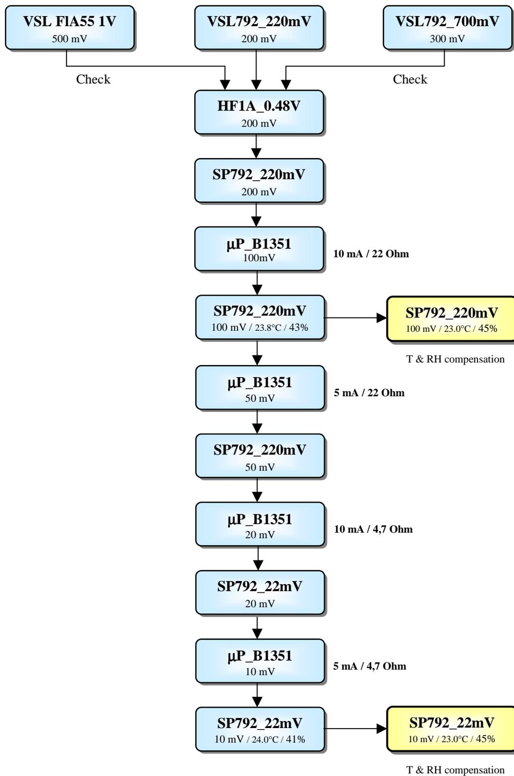
Figure 5. Step-down procedure of the low voltage AV-DV measurements via Ballantine 1351.
