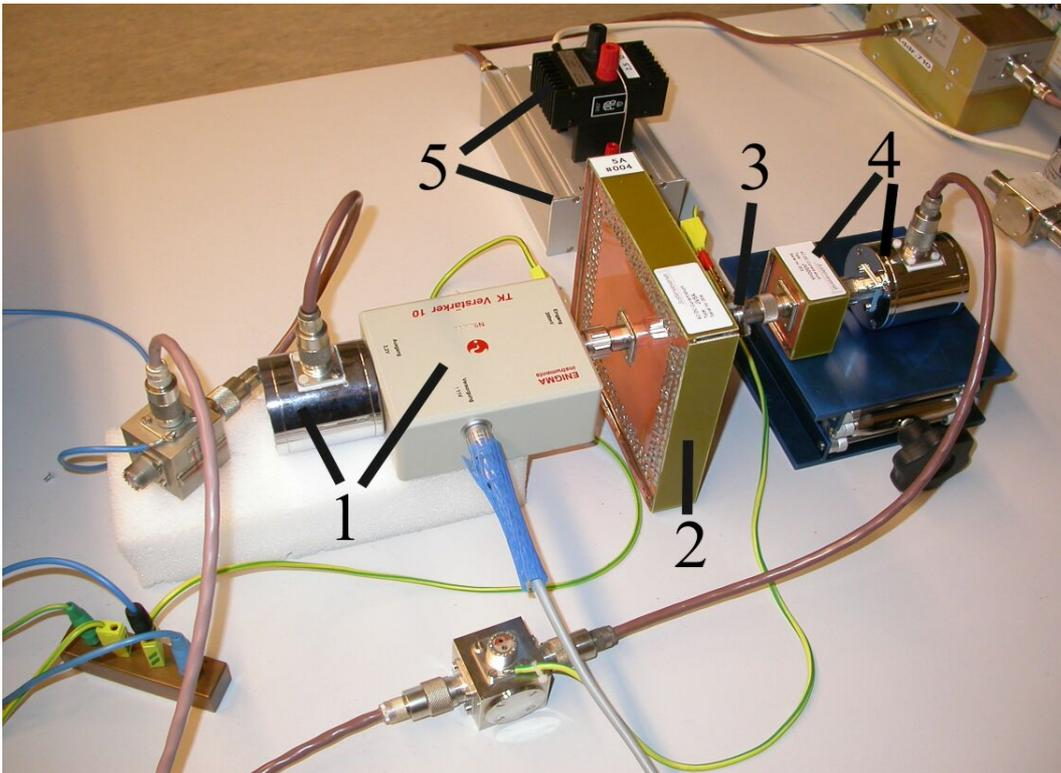
Fig. 2: PMJTC with amplifier (1), discrete  $\mu$ pot with 0.2- $\Omega$ -shunt (2), current Tee-connector (3), 1-A-shunt and PMJTC (4), 1 A/1 MHz transconductance amplifier with external shunt (5).
