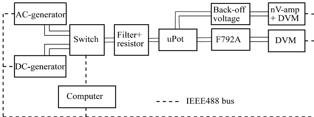
Fig. 2. Automated measuring system for comparison of micropotentiometer and Fluke 792A.
