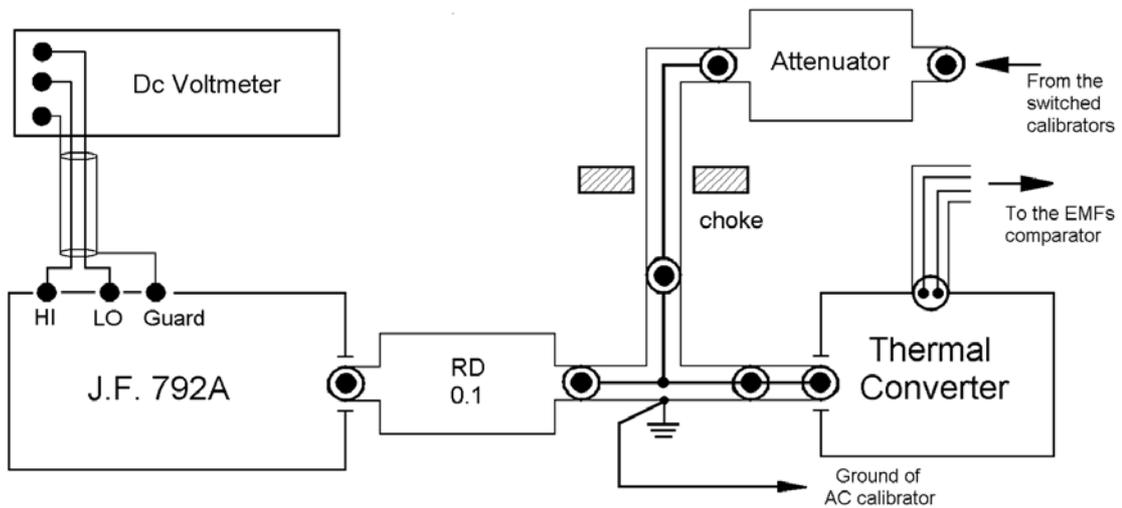
**Fig. 2** Scheme of the connection of the standards for 10 mV measurement.
