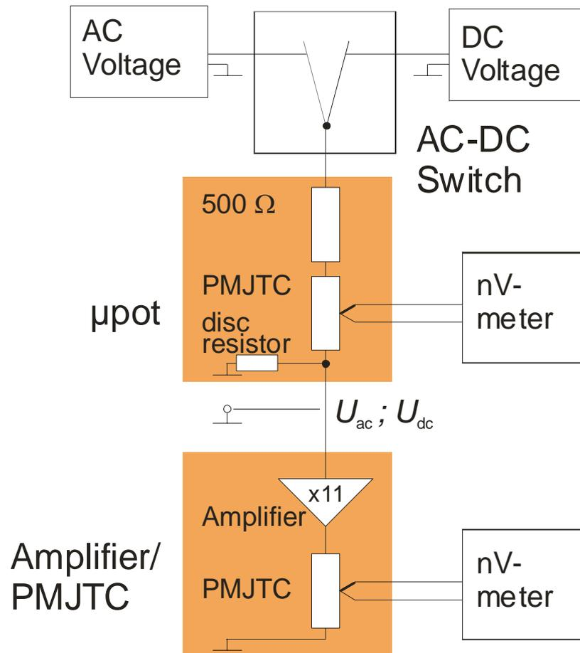
Fig. 1. Measurement set-up for AC-DC mV-transfer with common 10-mA  $\mu$ pots. With discrete  $\mu$ pots a transconductance amplifier as a current source is used and the 500- $\Omega$  resistor in the  $\mu$ pot is not needed.
