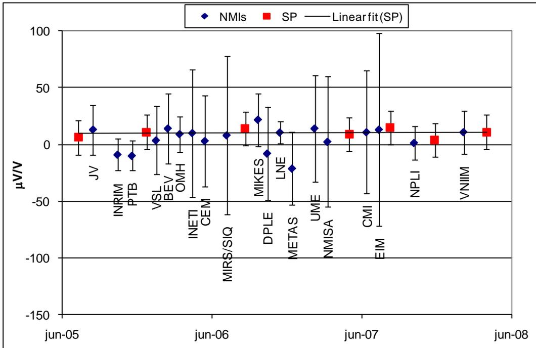
Figure 6 Reported values  $\delta_i$ , 10 mV, 1 kHz, and stability of travelling standard
