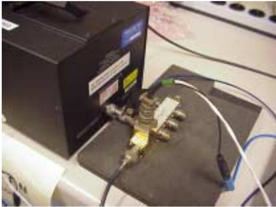
Figure 2 shows the set-up of the measurements between the Holt 12 en de SP\_Fluke 792A. A special N-male to N-male is used to connect the central ground.
