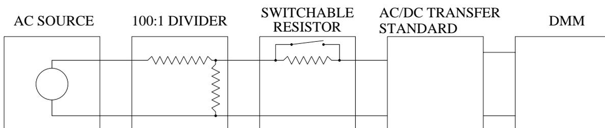
Figure 6: Input impedance measurement setup.
