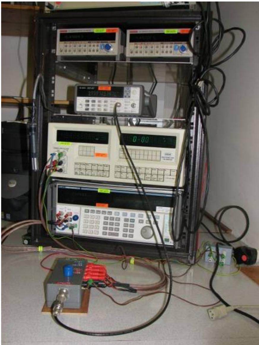
Figure 3: Frequency accuracy measurement setup.
