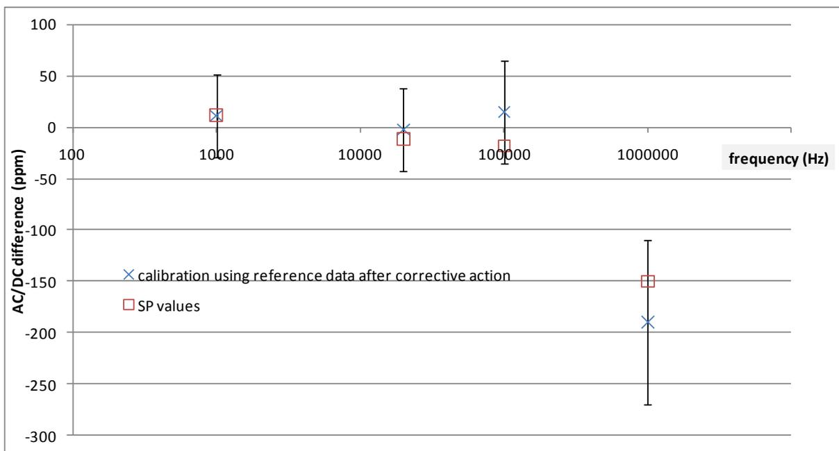
Figure 3: calibration of travelling standard at 10 mV: comparison of the values obtained by SP (squares) and of the METAS measurement during EM-K11 done with own's 792 A (crosses). The calibration values of METAS' own instrument are those obtained in 2010. Error bars correspond to METAS uncertainty (k=2)
