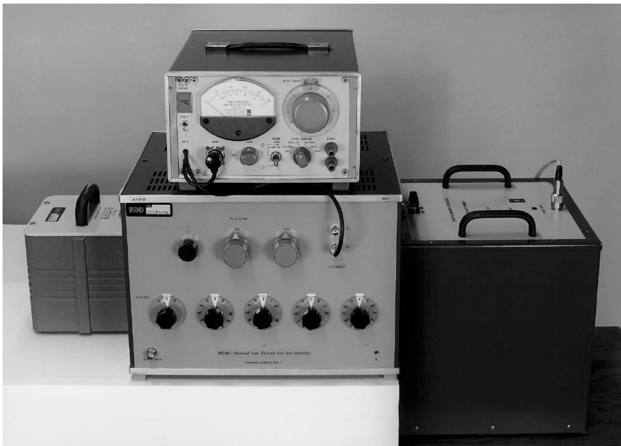
Figure 6: Pictorial view of the inductive voltage divider bridge
