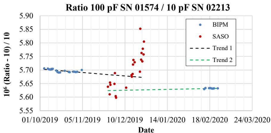
**Figure 5 Ratio of capacitors 100pF SN 01574 / 10 pF capacitor SN 01227.**
