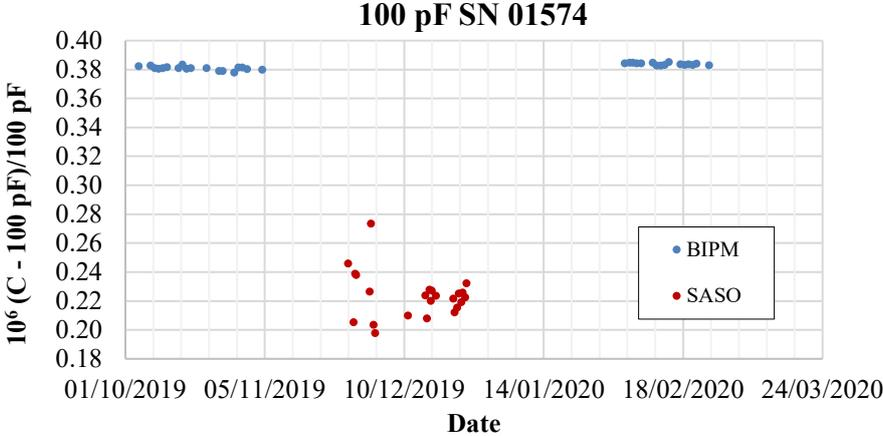
**Figure 1 BIPM and SASO measurements for the 100 pF capacitor SN 01574.**
