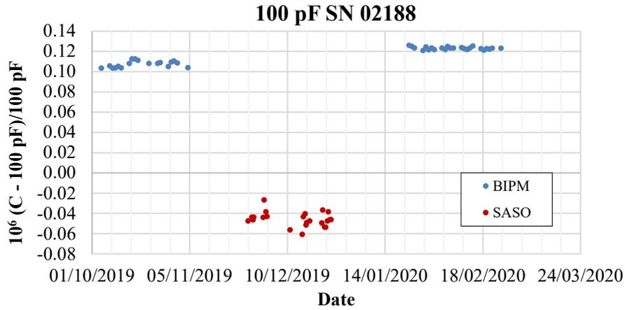
Figure 2 BIPM and SASO measurements for the 100 pF capacitor SN 02188.
