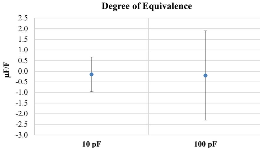
**Figure 7 Degree of equivalence between the BIPM and the SASO for 10 pF and 100 pF capacitance measurements and associated uncertainty ( $k = 2$ ).**
