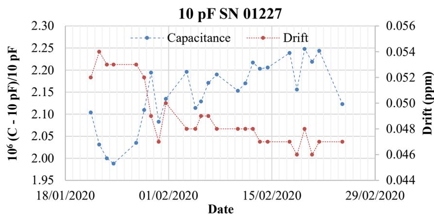
**Figure 6 Correlation of the capacitance value and 'drift' of the 10 pF capacitor SN 01227.**
