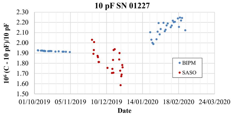
**Figure 4 BIPM and SASO measurements for the 10 pF capacitor SN 01227.**
