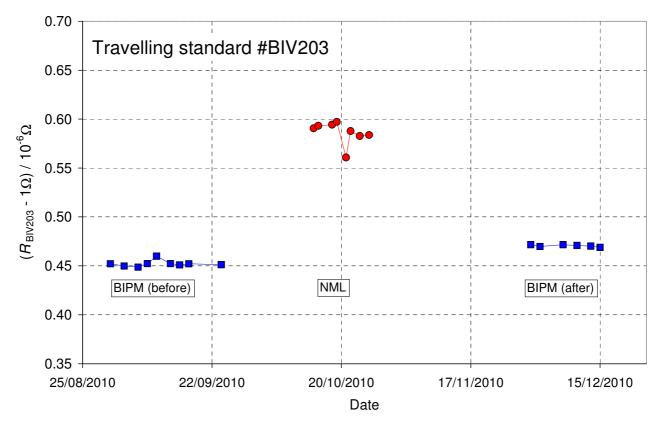
Figure 2: Calibrations at the BIPM (squares) and at the NML (circles) of the travelling standard ref. BIV203, expressed as the relative deviation from the nominal 1  $\Omega$  value.
