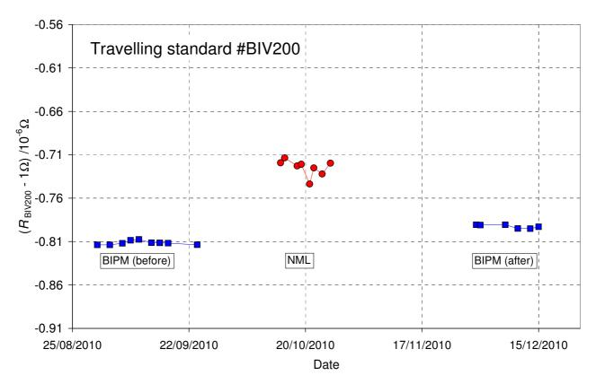
Figure 1: Calibrations at the BIPM (squares) and at the NML (circles) of the travelling standard ref. BIV200, expressed as the relative deviation from the nominal 1  $\Omega$  value.
