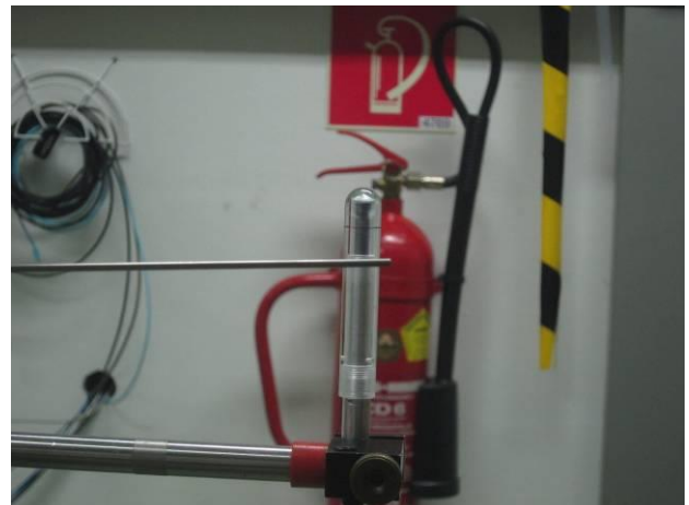
Figure 17 Air Kerma, therapy level Co-60, ionization chamber PTW T30012 including temperature sensor
