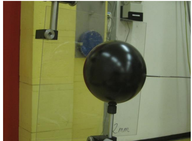
Figure 20 Air Kerma, radiation protection level Cs-137, ionization chamber PTW 32002 1 I, including 2 mm PMMA plate and temperature sensor
