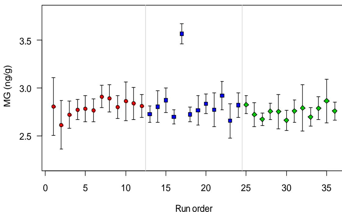
**Figure 3.** MG homogeneity in material CCQM-K85 as determined by exact matching IDMS performed on 12 samples in triplicate (2g sample size). The different colors indicate analysis performed on different days. Error bars represent the standard deviation.
