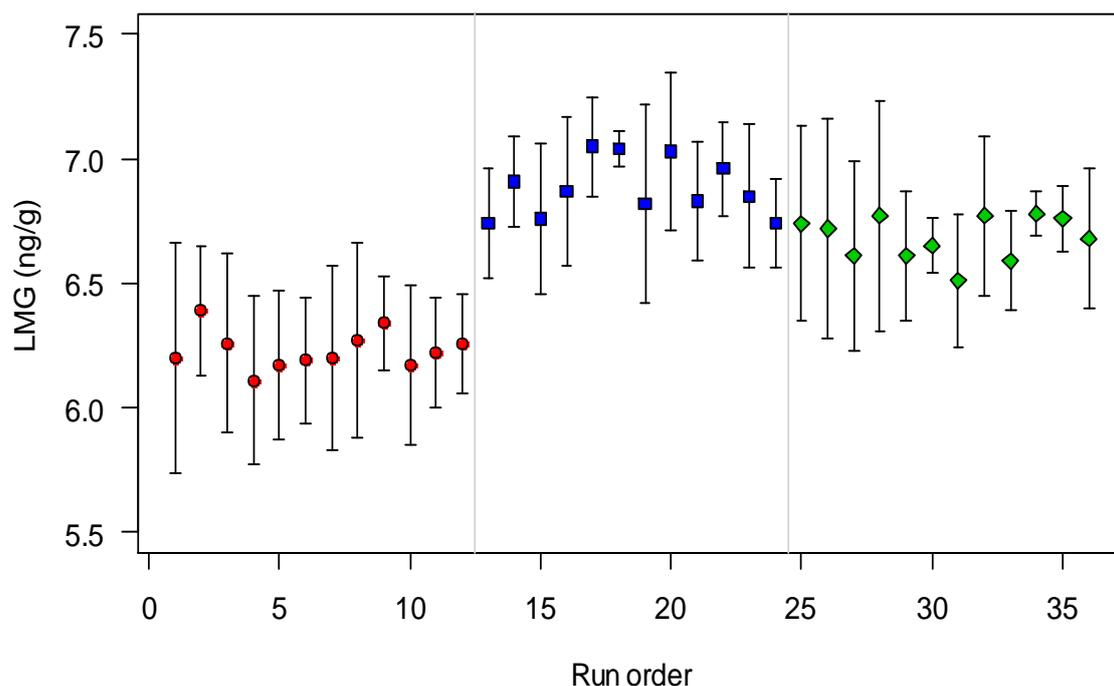
**Figure 4.** LMG homogeneity in material CCQM-K85 as determined by exact matching IDMS performed on 12 samples in triplicate (2g sample size). The different colors indicate analysis performed on different days. Error bars represent the standard deviation.
