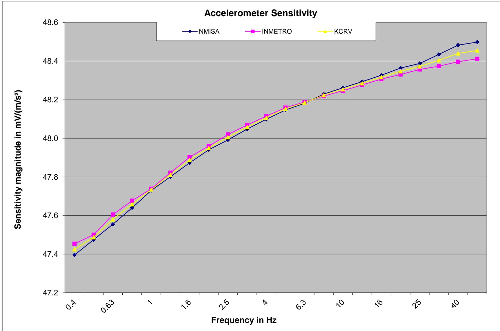
Figure 1: Sensitivity magnitude frequency response of the accelerometer standard as reported in tables 2 and 3
