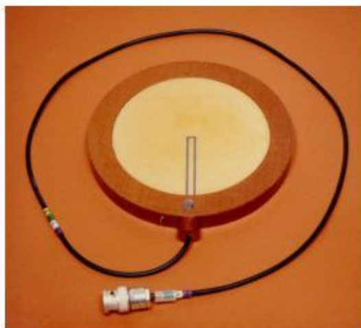
Figure 1: Photograph of a Marconi bilaminar membrane hydrophone of the type which will be used within the key comparison. The outside diameter of the supporting ring is 130 mm.
