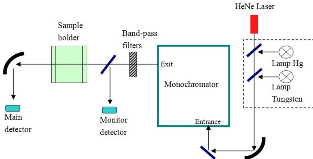
Table B5. Details of NIM's Measurement Setup
