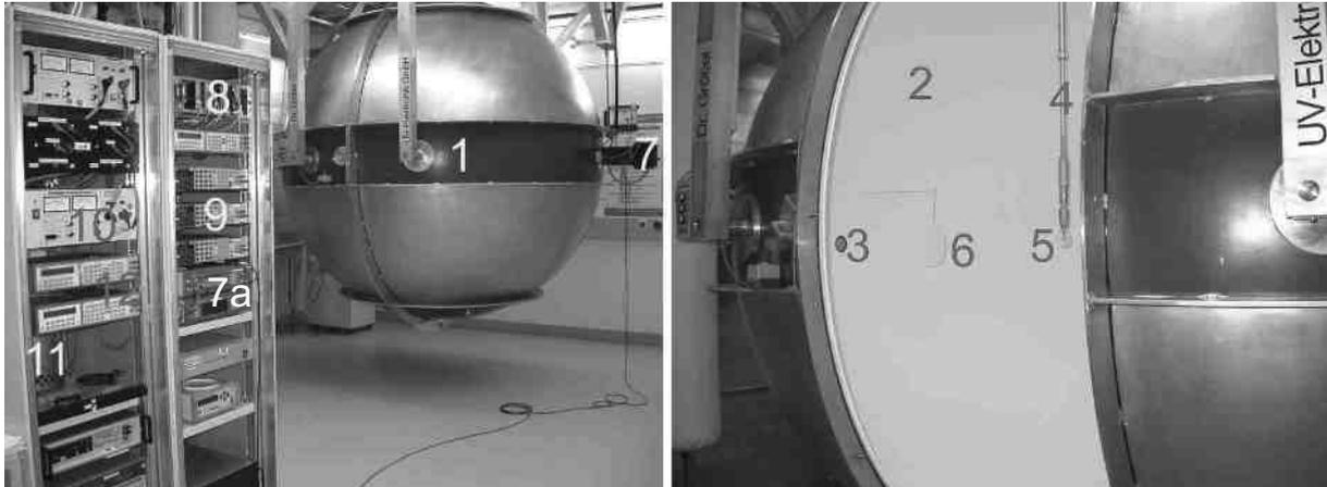
**Fig. 1, integrating sphere, 2.5 m diameter**
