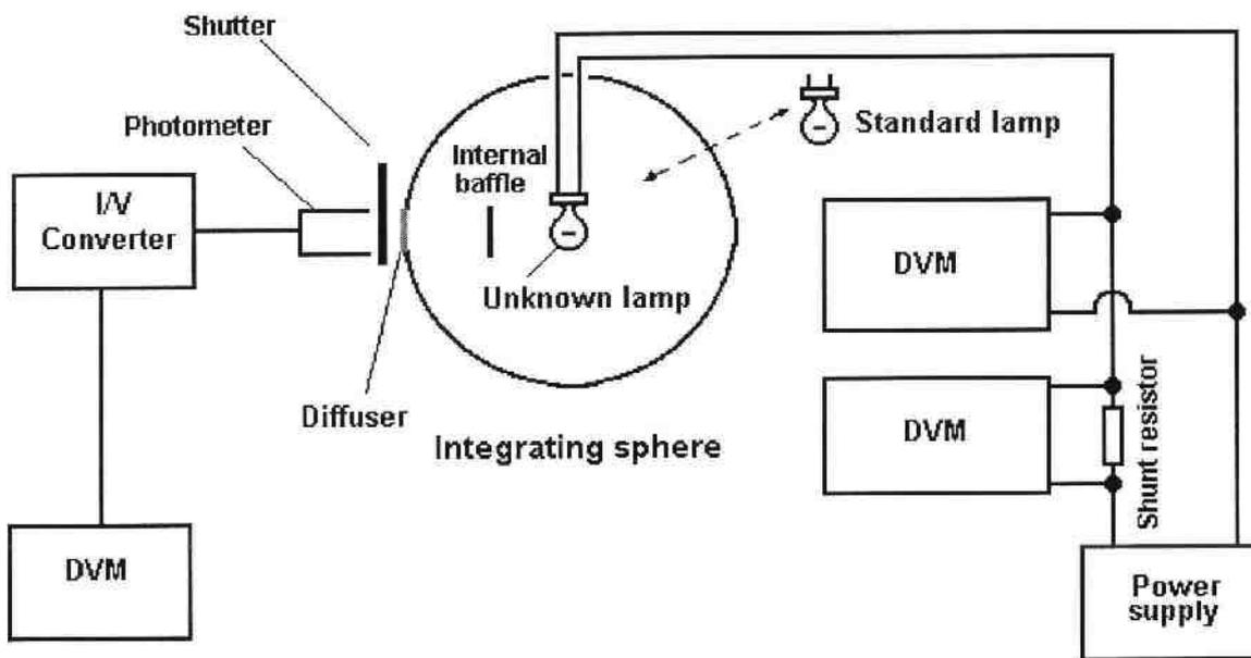
Fig. 1 Luminous flux transfer installation at INM
