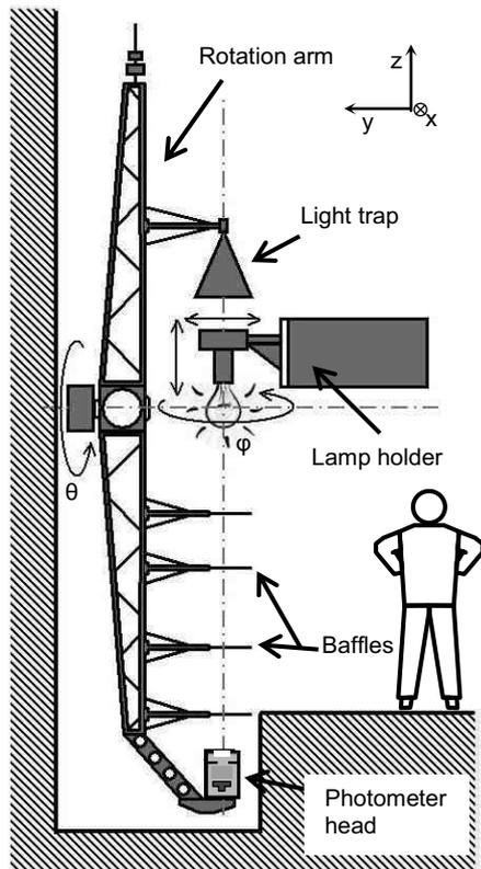
Figure 1: general view of the goniophotometer.: the lamp holder allows the alignment and the rotation of the lamp. The photometer rotates thanks to the rotation arm. 4 baffles and a light trap are used to reduce the stray light. The man is 1.80m.
