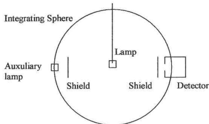
Picture 1.: Scheme of measuring setup
