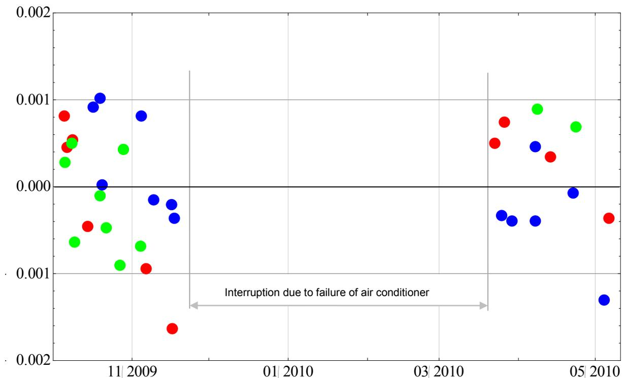
Fig. 3 Long term stability of responsivity of the integrating sphere verified by repeated measurements of three luminous flux monitor lamps (indicated by red, green and blue points) normalized to their mean luminous flux results
