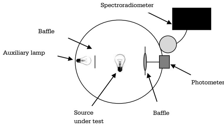
Figure 1: Top view schematic depiction of the 3 m sphere setup.
