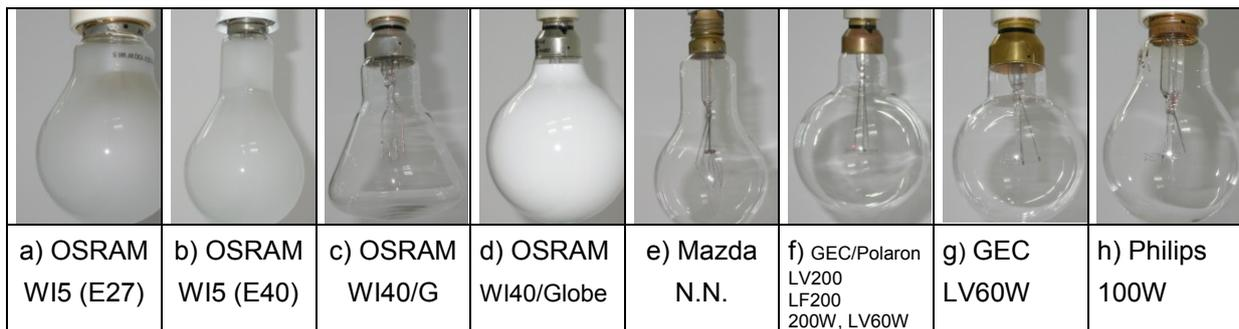
Fig. 1 Images of the eight different lamp-transfer-standards used by the participants identified by the manufacturers and the lamp types. If necessary the socket size is given in parentheses.
