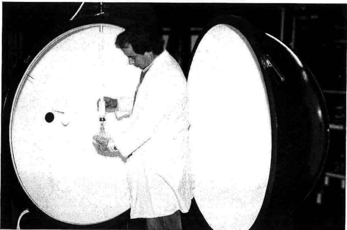
Fig.2 Photo of DMDM integrating sphere
