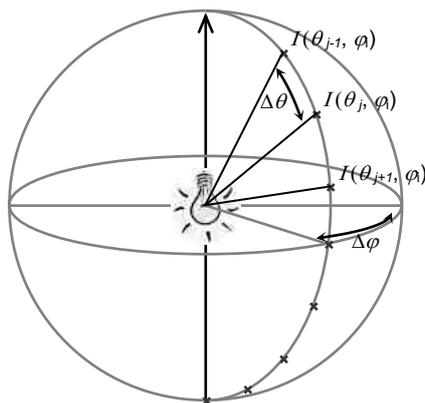
Figure 2: Angular notations.  $\theta$  is the elevation angle and varies between  $90^\circ$  and  $-90^\circ$ .  $\varphi$  is the azimuth angle.  $I(\theta_j \varphi_i)$  is the luminous intensity at the position  $(\theta_j \varphi_i)$ . For a luminous flux measurement, the steps are  $\Delta\theta = 3^\circ$  and  $\Delta\varphi = 6^\circ$  which given 3600 luminous intensity measurements
