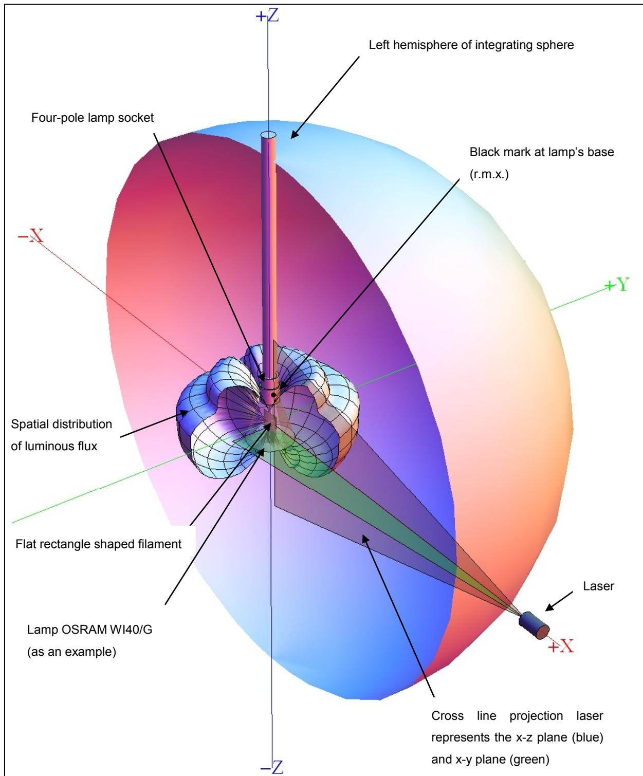
Fig. 2: Example of the mechanical alignment of the lamps for rotation and height inside the integrating sphere.
