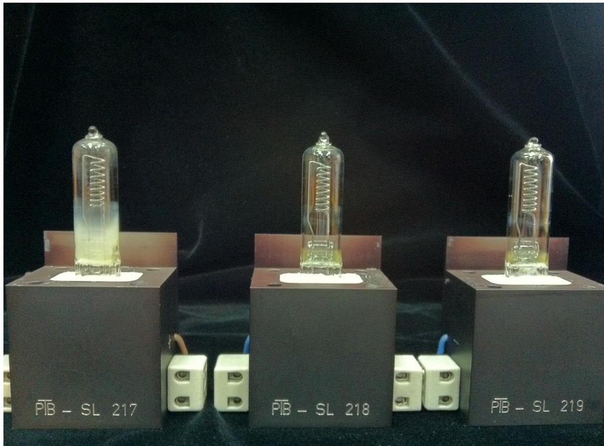
**Figure 47. Photograph of lamps measured by VNIIOFI; note white deposit at base of lamp SL 217.**
