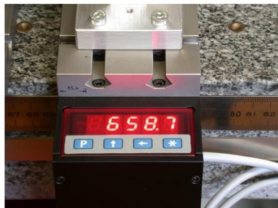
**Figure 39. Absolute encoded magnetic ruler**
