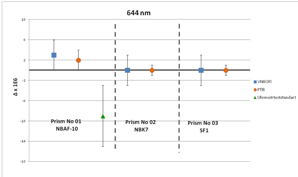
Figure 4.6. Difference from CRV ( $\Delta_i$ ) with expanded uncertainties  $U(\Delta_i)$  at 644 nm.
