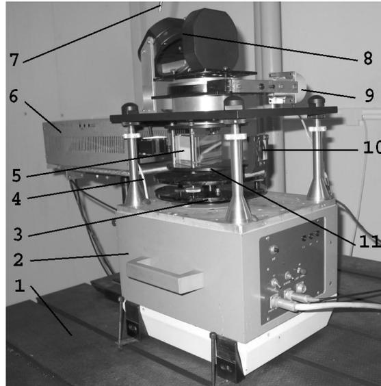
Fig. A.1.1. VNIIOFI facility for refractive index measurement: 1 – table; 2 – dynamic goniometric spectrometer DG-1L; 3 – mirror rotating stage; 4 – optical fiber; 5 – triangular glass prism; 6 – interferometric null-indicator; 7 – air temperature detector; 8 – mirrors; 9 – stepping motor rotates the stage; 10 – two-sided mirror; 11 – prism stepping rotating stage.
