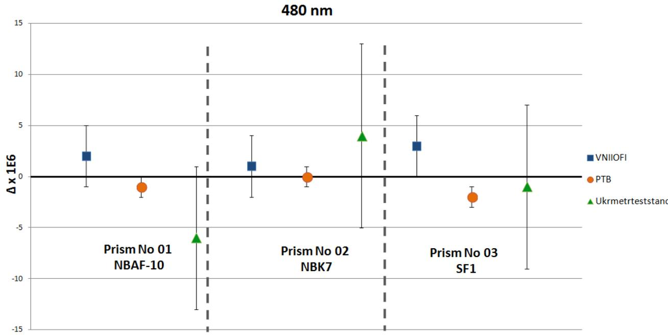
Figure 4.1. Difference from CRV ( $\Delta_i$ ) with expanded uncertainties  $U(\Delta_i)$  at 480 nm.
