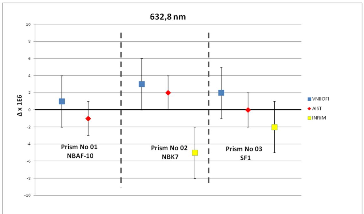
Figure 4.5. Difference from CRV ( $\Delta_i$ ) with expanded uncertainties  $U(\Delta_i)$  at 632.8 nm.
