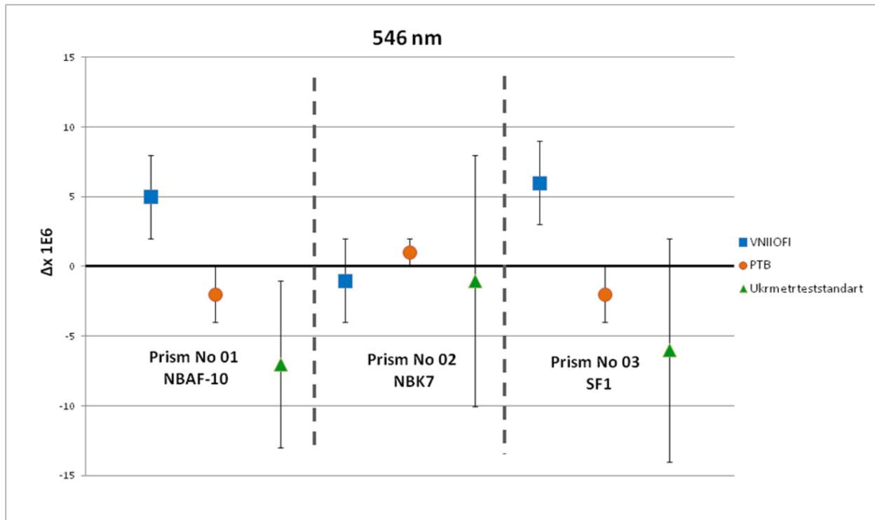
Figure 4.3. Difference from CRV ( $\Delta_i$ ) with expanded uncertainties  $U(\Delta_i)$  at 546 nm.
