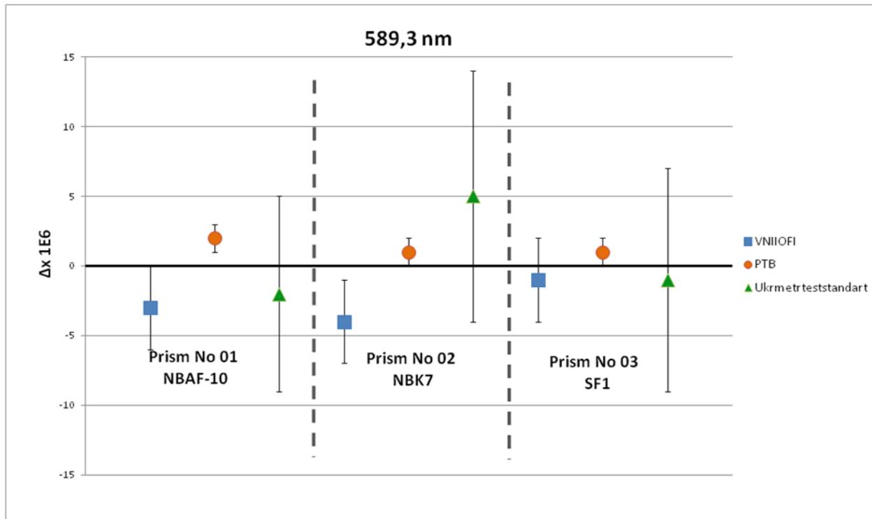
Figure 4.4. Difference from CRV ( $\Delta_i$ ) with expanded uncertainties  $U(\Delta_i)$  at 589.3 nm.
