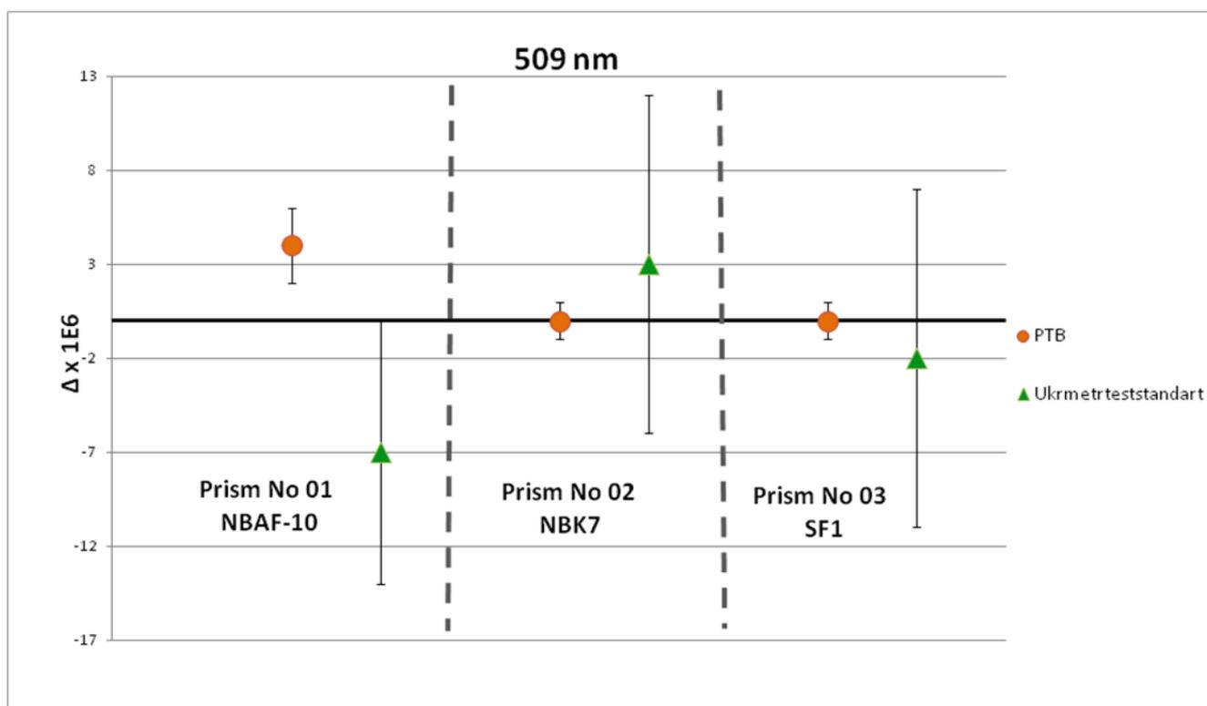
Figure 4.2. Difference from CRV ( $\Delta_i$ ) with expanded uncertainties  $U(\Delta_i)$  at 509 nm.
