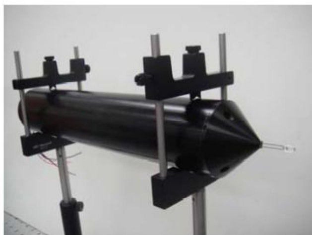
Fig. 4-40. Photograph of an LED mounted on the cylindrical LED mount in NIST.
