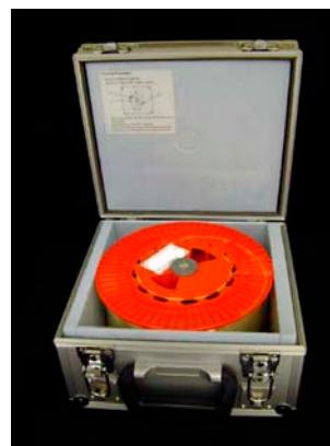
Fig. 1. Reference Fibres mounted in a thermal enclosure.
