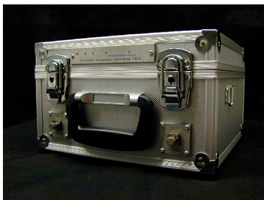
Fig. 1. Reference Fibres mounted in a thermal enclosure.
