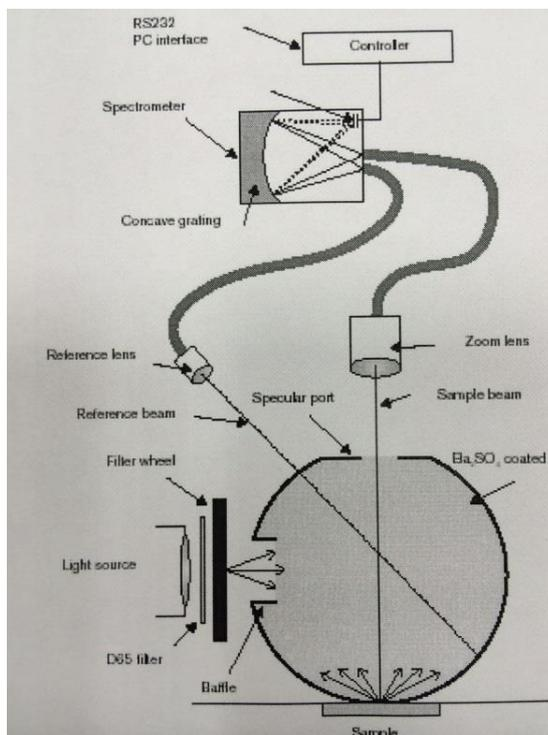
Figure A2.3. Structural diagram of the spectrophotometer ELREPHO 071
