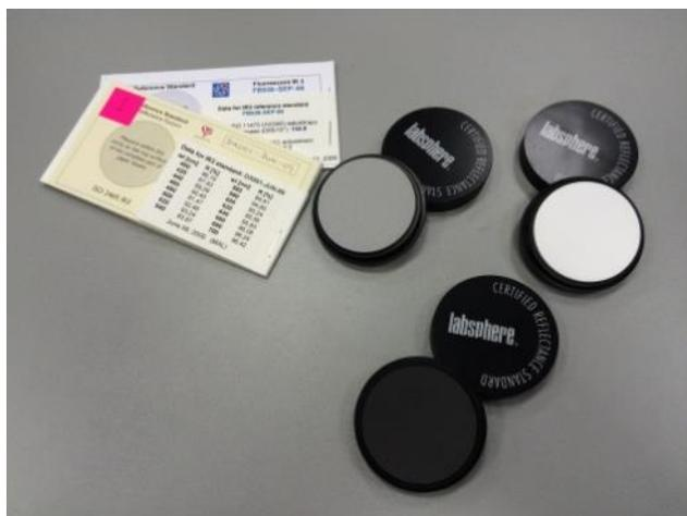
Figure A2.2. Standard samples used at BelGIM to calibrate the spectrophotometer
