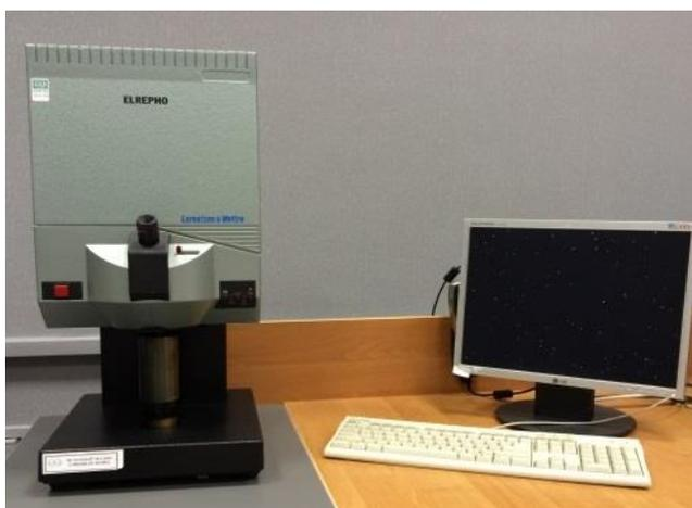
Figure A2.1. ELREPHO 071 spectrophotometer appearance
