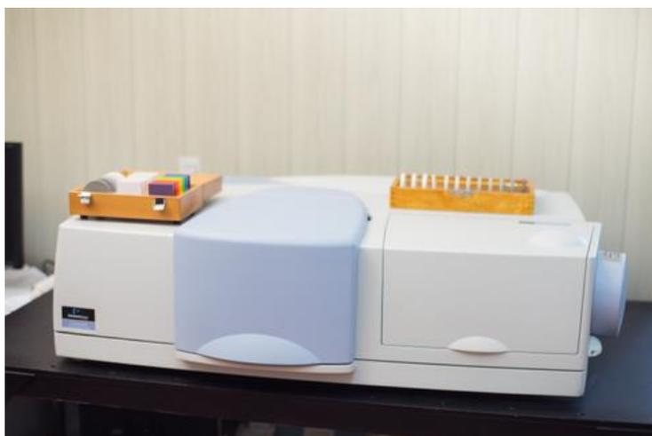
Figure A1.1. Lambda 850 spectrophotometer appearance
