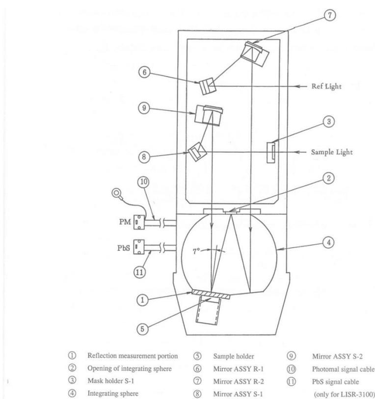
Fig. B.1. Structure of integrating sphere and accessories for reflection measurements
