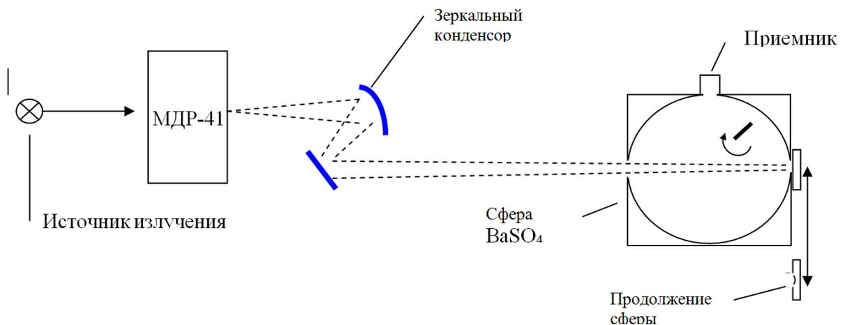
Figure A3.3. Scheme for measuring the spectral coefficients of diffuse reflection applied in the National primary standard facility of Ukraine
