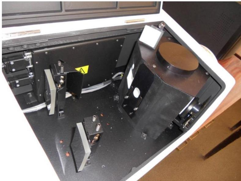
Figure A3.2. Internal structure of the Spectrophotometer Lambda 950
