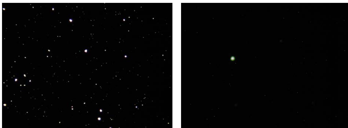
Fig. 9 Low magnification optical dark-field images of diode A2 after return from NIST (left) and diode AXUV#5 stored at PTB (right). The field shown is 1.2 mm by 1.6 mm in the centre of the diode.
