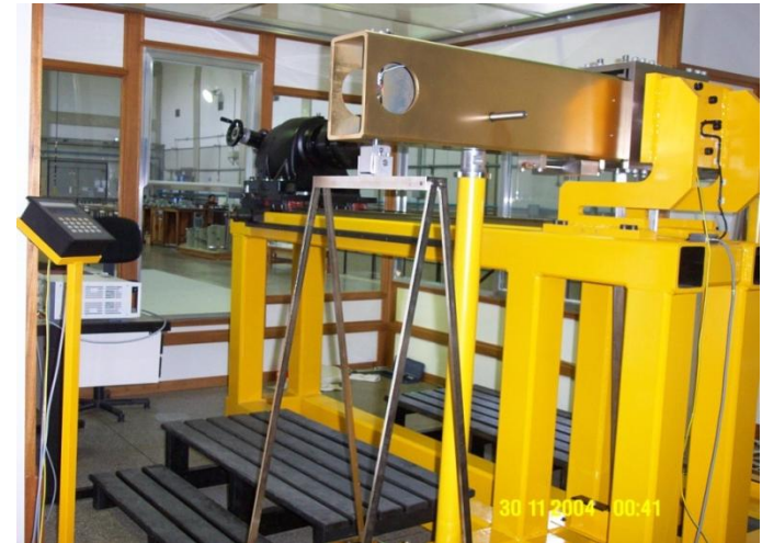
Dead weight torque machine of INMETRO 1 N·m up to 3 kN·m
