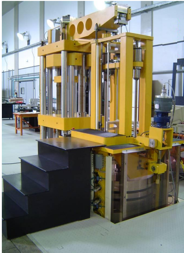
Dead weight force machine of INMETRO 100 kN direct, 1000 kN transfer
