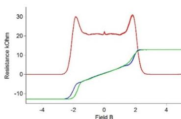
Figure 1. **A.** Sample gated using only chemical gating shows well-defined quantization at 2K. The polymer spacer thickness is such that the doping at 2K reaches  $n = 2 \cdot 10^{11} \text{ cm}^{-2}$  electrons. Mobility exceeds  $7000 \text{ cm}^2/\text{Vs}$ .
