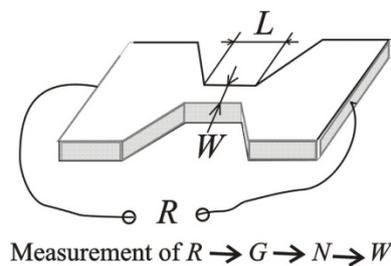
Fig. 1 Estimations of the width of a nanostructure by electrical measurements (R – resistance, G- conductance, N – number of transmission channels, W – width).
