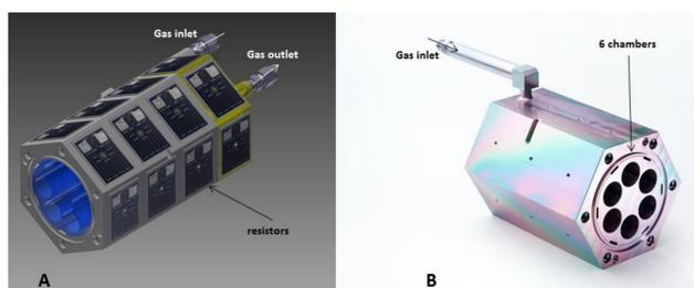
Figure 2: Computer-Aided Design (A) and picture (B) of the in-house developed oven of ReGaS2 with 6 permeation chambers. One chamber is reserved for the internal temperature sensor. The oven is entirely coated with SilcoNert®2000.
