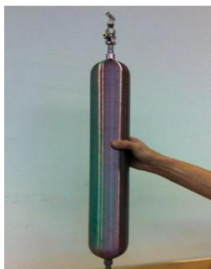
Figure 5: Picture of novel coated stainless steel cylinder used for preparation of VSL reference gas mixtures.
