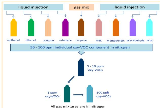
Figure 6: Preparation scheme of VSL reference gas mixtures for oxygenated VOCs. Preparation method: gravimetric according to ISO 6142-1:2015.
