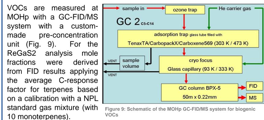
Figure 9: Schematic of the MOHp GC-FID/MS system for biogenic VOCs
