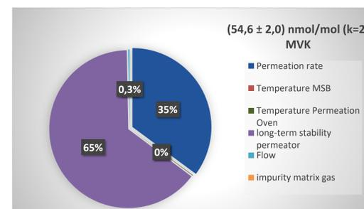
Figure 4: Uncertainty budget for the generation of circa 54 nmol/mol methyl vinyl ketone (MVK) with the ReGaS2 during several days. The main contributions to the uncertainty come from the permeation rate determination and its long-term stability.
