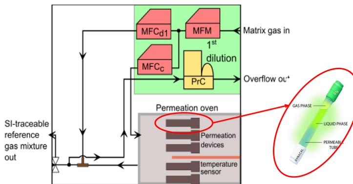
Figure 1: Design of the mobile SI-traceable reference gas generator «ReGaS2». On the right-hand side, as example for the permeation device, a sketch of a typical tubular permeator.
