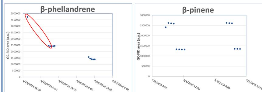
Figure 10 and 11: Measurements of β-phellandrene and β-pinene with GC-FID generated with ReGaS2 at 2 different concentrations by changing the dilution flow. Figure 10 : 10 - 7 nmol/mol of β-phellandrene . Figure 11 : 50 - 30 - 50 - 30 nmol/mol of β-pinene. The red circle shows the stabilisation periode of the permeator.
