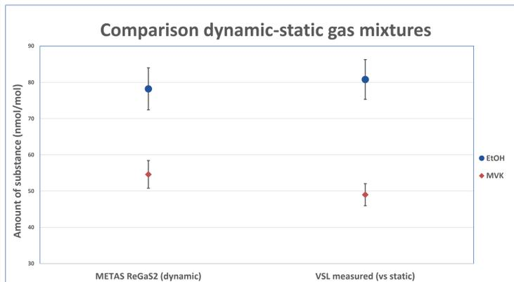
Figure 7: Comparison of Ethanol and Methyl Vinyl Ketone (MVK) produced dynamically with ReGaS2 (METAS) and gravimetrically in novel cylinders (VSL). The blue and red dots are the amount of substance fraction of Ethanol and MVK respectively. Error bars represent uncertainties (k=2)
