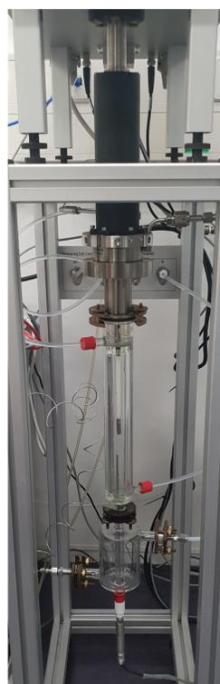
Primary gravimetric dynamic gas standard based on permeation
