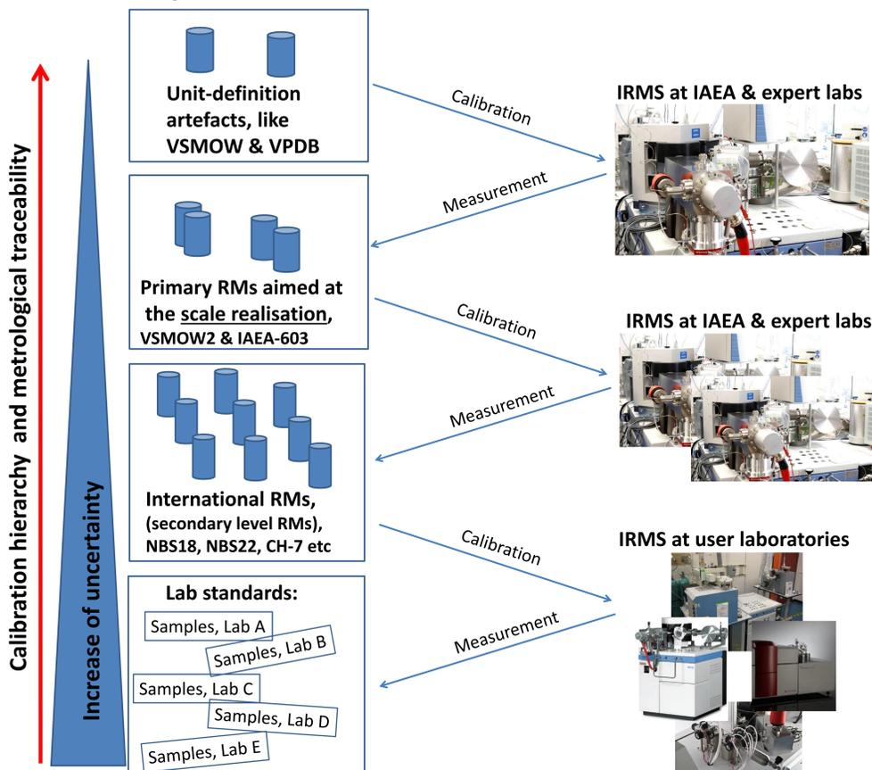
Each additional measurement step increases the combined uncertainty. Note, RM producers have the same instruments as end-users.
