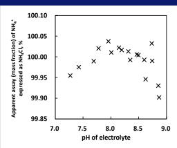
Dependency of NH<sub>4</sub>Cl assays on pH. The assays had a maximum around pH 8.0 to pH 8.5. The lower assays were understood as a result of the evaporation of NH<sub>3</sub> at higher pH values and the insufficient BrO electrogeneration (e.g., Br<sub>2</sub> generation) at lower pH values.
