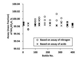
Homogeneity test for NH<sub>2</sub>SO<sub>3</sub>H. Ten bottles were chosen from 400 bottles for the homogeneity test. Both NH<sub>4</sub><sup>+</sup> and H<sup>+</sup> were determined by coulometric titration.
