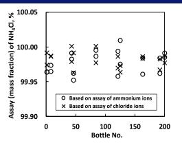
Homogeneity test for NH<sub>4</sub>Cl. Ten bottles were chosen from 200 bottles for the homogeneity test. Cl- were determined by gravimetric titration with AgNO<sub>3</sub> standardized based on NMIJ CRM NaCl through precipitation reaction.
