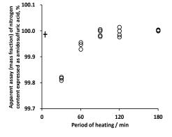
Decomposition of NH<sub>2</sub>SO<sub>3</sub>H with H<sub>2</sub>SO<sub>4</sub> by heating. NH<sub>2</sub>SO<sub>3</sub>H seemed to be completely decomposed more than 90 min by heating; the assays were close to 100 %. The bar on the left indicates the certified value (k = 2) of NH<sub>2</sub>SO<sub>3</sub>H as an acid determined by coulometric titration with electrogenerated OH-
