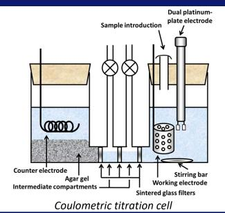
Coulometric titration is one of the primary methods of measurement, and provides the link to the SI by measuring the electric charge (electrical current and time) in an electrochemical reaction based on Faraday's Laws of electrolysis.
