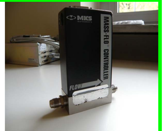
Fig 1: INRIM MKS Mass Flow Controller
