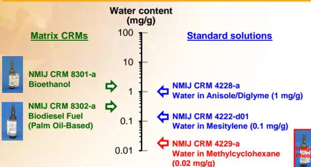
The CRMs for water content are virtually impossible to use after dilution since they are affected by water contained in the diluent and water absorption and/or desorption during preparation. Therefore, these CRMs at each required concentration level must be supplied.
