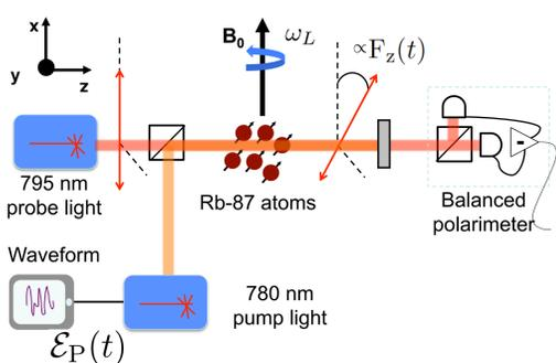
A waveform, carried by an optical field, is mapped onto the collective spin orientation of an ensemble of  $N$  ground state alkali atoms:
