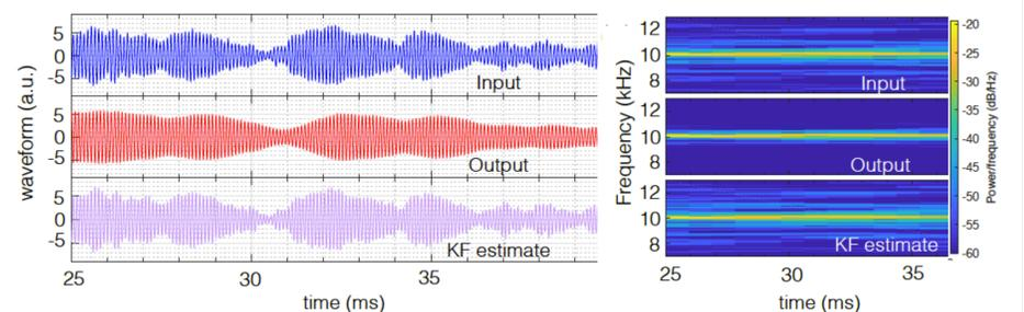
Left: a representative applied waveform (input) along with the corresponding measured angle (output) and the recovered waveform (KF estimate).
