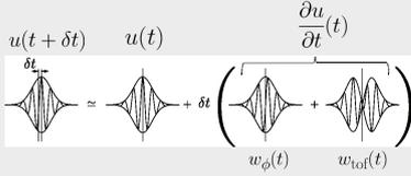
Enhancement of accuracy using the complete detection mode in homodyne detection [3]
