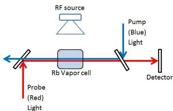
Figure 1. Schematic diagram of the setup considered for E-field measurement with the help of EIT and ATS
