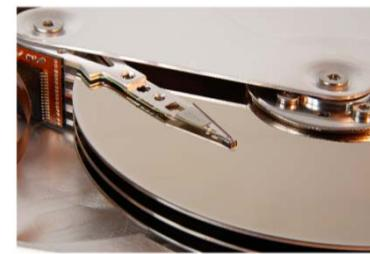
*Typical seek time for acceleration and deceleration of read heads is 4 ms.*
