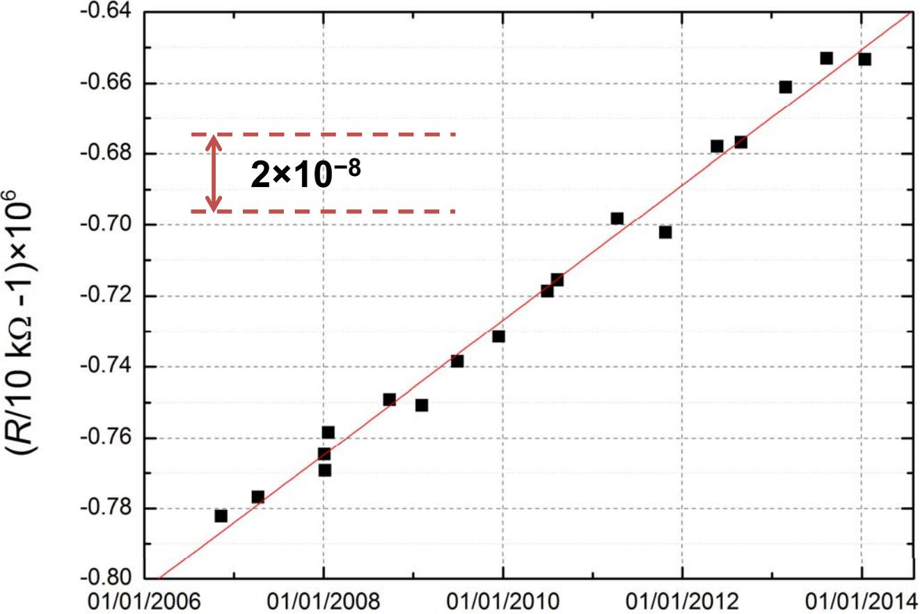
Example of a 10 kΩ working standard maintained at the BIPM – measurements against the QHR over last 10 years
