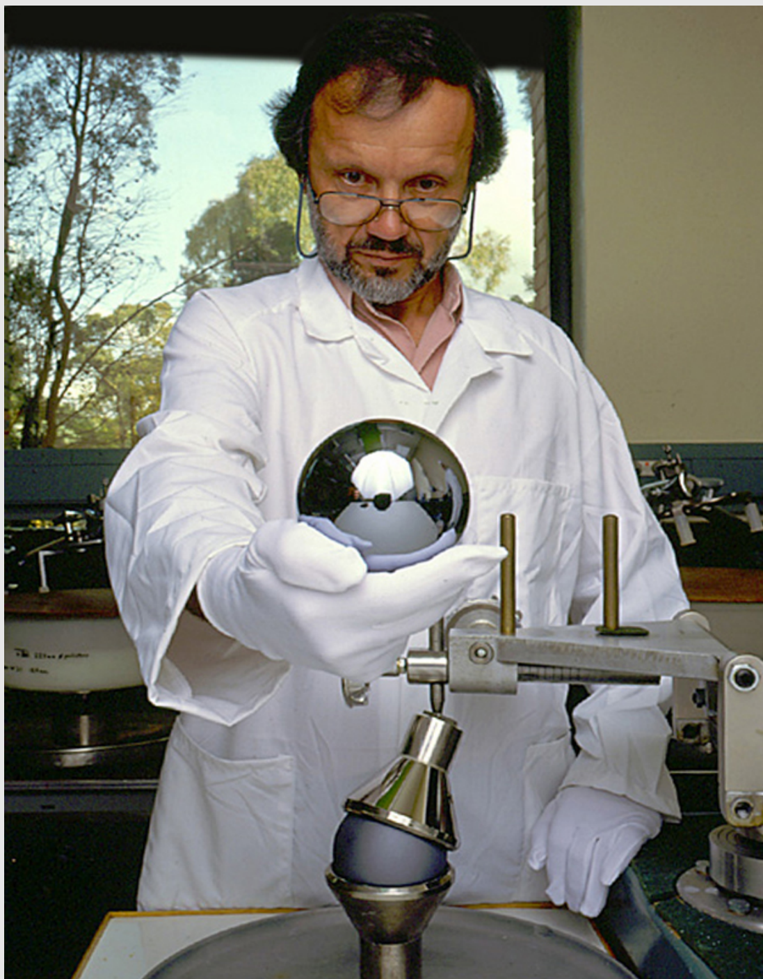
"Silicon sphere for Avogadro project" by The Commonwealth Scientific and Industrial Research Organisation of Australia - CSIRO.
