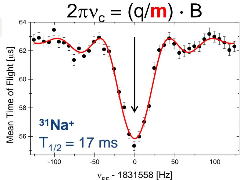
Mass determination via cyclotron-frequency determination
