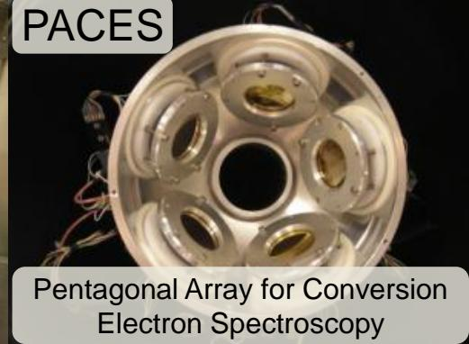
Pentagonal Array for Conversion Electron Spectroscopy
