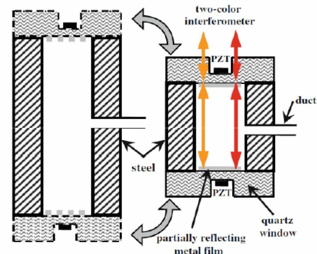
Fig. 1 Schematic diagram of two fixed-length, cylindrical, cavity resonators with interchangeable ends
