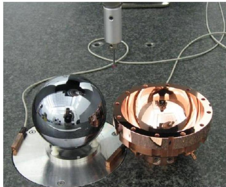
**Figure 3.** CMM measurements conducted at NPL probing the inner surface of a copper quasi-sphere alongside a spherical density and volume standard. Note the two thermometers (embedded in copper blocks) positioned around the artefacts.
