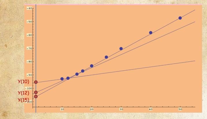
Step #2: set of data y(x) is plotted and fitted again. The procedure may be repeated iteratively.
