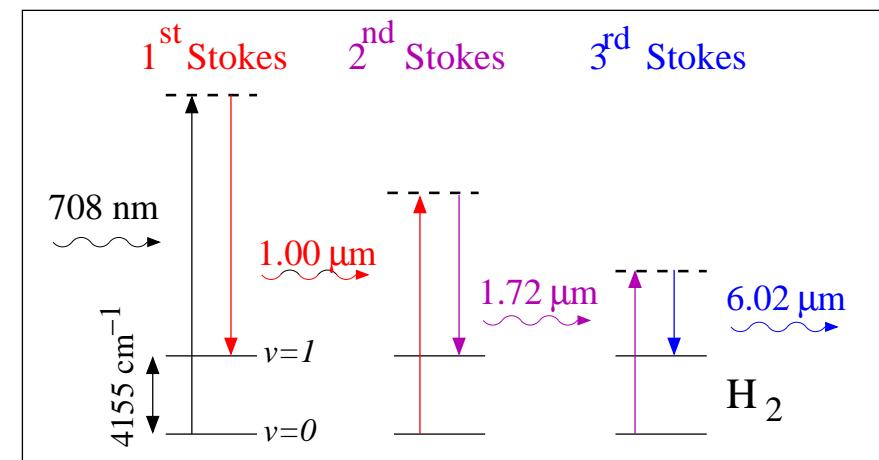
$v^{6\mu m} = v^{708nm} - 3 \cdot \hbar \omega_{vib}$
