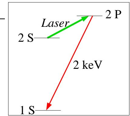
normalize  $\frac{\text{delayed } K_{\alpha}}{\text{prompt } K_{\alpha}}$   $\Rightarrow$  Resonance
