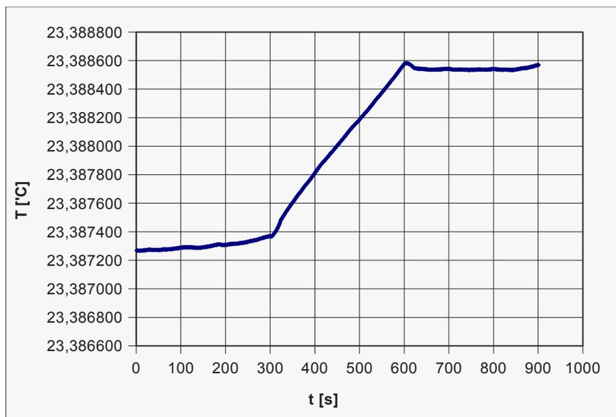
Fig. 11. Example of temperature rise measurement for the BIPM250 x-ray beam (first test)
