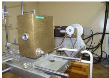
Fig. 1. The primary standard for air-kerma of the GUM for low energy x-ray ranges on irradiation bench
