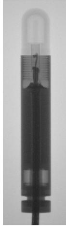
Fig. 7. The assembled a ionization chamber IGNAŚ-IC16#001 (radiography)
