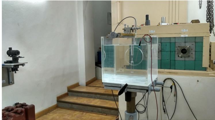
Fig. 8. The secondary standard of absorbed dose to water of the GUM for  $^{60}\text{Co}$  on irradiation bench
