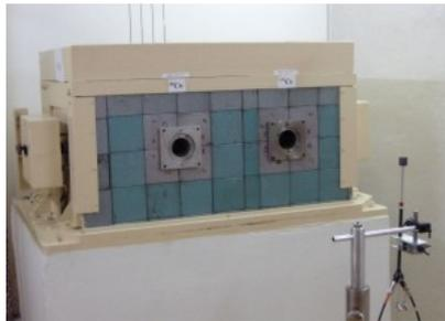
Fig. 5. The primary standard of air kerma of the GUM for  $^{60}\text{Co}$  and  $^{137}\text{Cs}$  (a ionization chamber type ND 1005/A, serial number 8303) on irradiation bench
