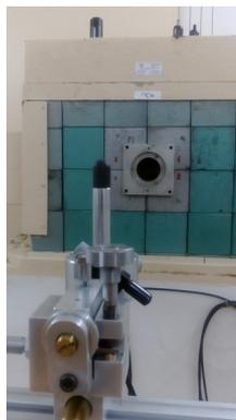
Fig. 6. The new primary standard of air kerma of the GUM for  $^{60}\text{Co}$  and  $^{137}\text{Cs}$  (a ionization chamber IGNAŚ-IC16#001) on irradiation bench
