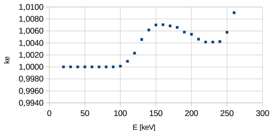
Fig. 3. Calculated electron-loss correction factor for the GUM medium-energy free-air chamber standard in EGSnrc (FAC code)
