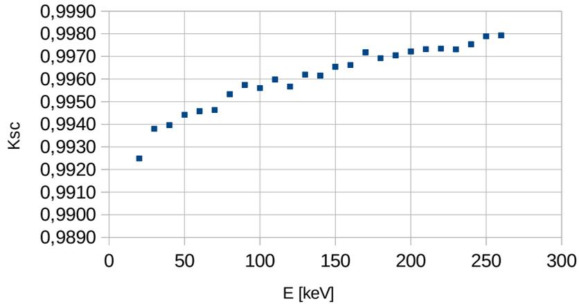
Fig. 4. Calculated photon-scatter correction factor for the GUM medium-energy free-air chamber standard in EGSnrc (FAC code)
