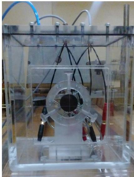
Fig. 9. First version of the assembled graphite calorimeter of the GUM
