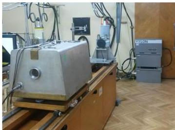
Fig. 2. The primary standard of air-kerma of the GUM for medium energy x-ray ranges on irradiation bench
