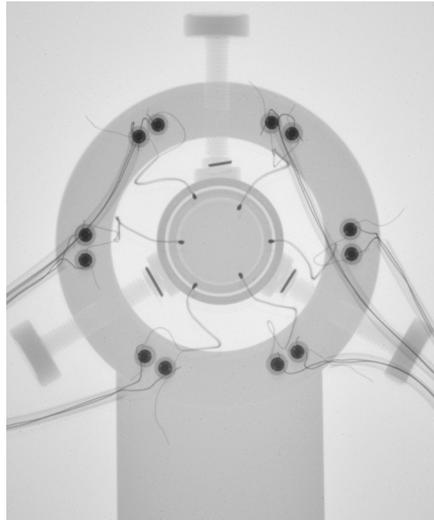
Fig. 10. First version of the assembled graphite calorimeter (radiography)
