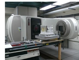
BIPM calorimeter mounted on the patient couch of the NIST clinical accelerator
